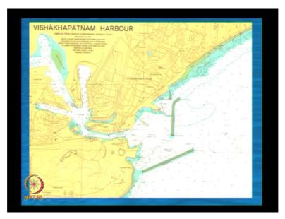
It shows the layout for Visakhapatnam harbour, both inner harbours, turning circle, entrance channel for the inner harbour and the outer harbour, breakwaters, fisheries harbour. This
