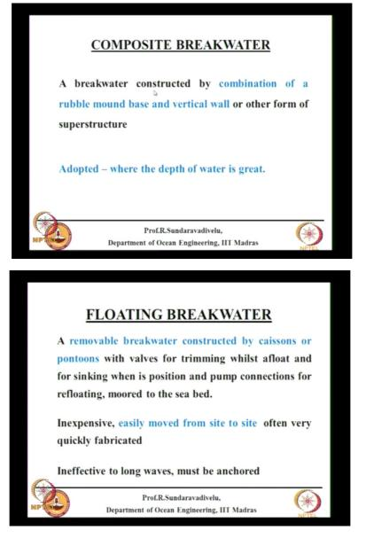
A composite breakwater is a combination of rubble mound base and vertical walls, besides vertical wall it can be others form of superstructure. This is adapted where the depth of water this more, more than 15 metres. Then we have other types of floating breakwaters, 2<sup>nd</sup> type of breakwater. The 3 types of breakwater rubble mound, caisson, composite, we can say 95 percent of the breakwater in the world, they are of that type. Whereas the other types, maybe 5 percent will be used.
