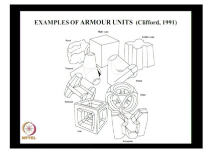
This is offshore breakwater, offshore breakwater means the top level is very close to the design water level. These are the various armour units, this is called as tetrapod, plain cube, this is natural rock, this is called as acropode, acropode is same as this only, but slightly different in shape. So these are the different samples.
