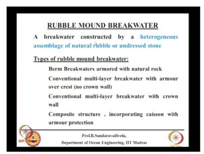
So now we will see rubble mound breakwater constructed by a heterogenous assemblage of natural rubble or undressed stone. Rubble means store only, undressed stone, undressed means you do not make it perfect. You go to temples and all, they make the size perfect, but perfect size is not good for rubble mound breakwater, you should not dust the stone, it should be random in shape. What is heterogenous, what is the literal meaning of heterogenous?
