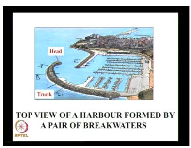
This shows layout of the breakwater, we always a pair of breakwater. And this is for a marina, in foreign countries we have marina where we have the pressure boats that are being used
