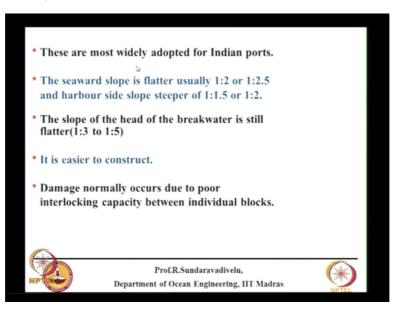
We will be concentrating more on rubble mound breakwater because this is the most widely adopted for Indian ports. Most of the ports, 99 percent most means, we have only rubble mound. I said there is a slope, Seaward look and the Harbourside slope, the Seaward slope is between 1 is to 2 or 1 is to 2.5 and Harbourside slope is 1 is to 1.5 to 1 is to 2. So in the 1<sup>st</sup> slide I have shown what is the seaside and what is the Harbourside. Seaside, the slope is
