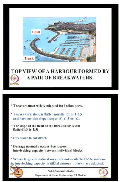
So this slope is 1 is to 3 to 1 is to 5, this slope is 1 is to 1.5, this slope is 1 is to 2, is it clear? This is the seaside, 1 is to 2, Harbourside 1 is to 1.5, in the head section it is 1 is to 3, 1 is to 3
