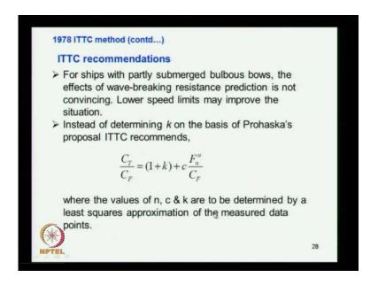
So, for ships with submerged bulbous bow the effect of wave breaking resistance prediction is not convincing. So, you that means hardly with hardly submerged bulbous bow, so we have to design the bulbous bow. And if it is partly submerged they estimation wave breaking resistance it is not convincing, because of the you know part of hidden wave creation you know bulbous bow is provided for reducing a wave breaking resistance. And I have already discussed when we discuss about bulbous bow effect.
