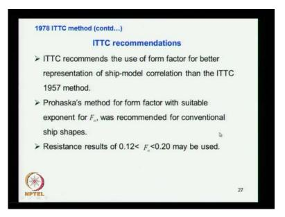
Suggested in the 1978 ITTC method, so ITTC recommends the use of form factor for better representation ship, in that is what we have seen 1978 method it shown compared
