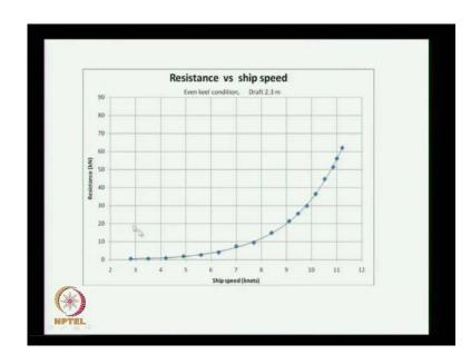
Then its plotted you get the resistance seconds speed you get the resistance curve. And then you have the R t into v that gives a effective power.
