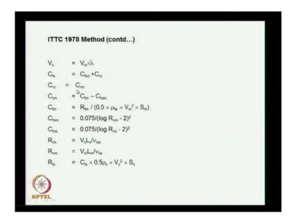
Then you have all this parameters are known, so finally get C rm is equal to C tm minus C fom and all this quantity is coming from that of the C fom of the model C f of the ship. And Reynolds sum are estimated and finally you have the quantity is here the model and.
