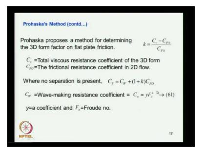
So, this are things we have seen representation of the wave making resistance as V power 6 of Froude number power raise to 6, and subsequently the wave resistance coefficient will be proportional to Froude number raise to 4.
