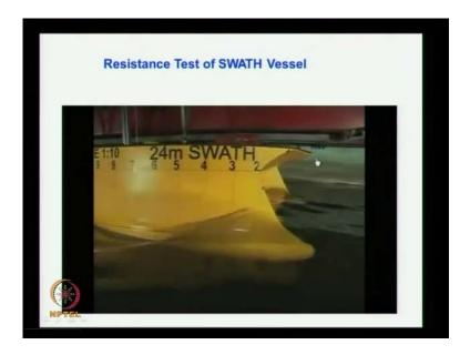
We tried different version of the and also different configuration of the Swath vessel and the you can see here in the middle there is a gap. This is actually 4 hulls 1 hull 1 hull here another hull here the same thing on the other side. And you can say the middle portion there is a gap, so there is a connection. So, it has been found that the middle region is creating lot of waste.
