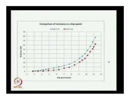
So, you plot effective power against the speed of the ship sp this is a effective power of the ship. Now, with the tests have been repeated for another draft for 2.5 metre, so this varies plotted here and this what is shown here. This is for the 2.5 metre higher draft and this is for allowance, so this test may be required when their case. When the ship is you know see more or may be a ship is design to have more displacement and when it
