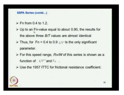
So, here the fluid number varies from point 4 to 1.2 up to a fluid number value of point results for above e B by T values of almost identical. So, that is what this is we have considered B by T value is 3.5 and 4 say is at up to point the Froude number of 0.9 where it is non dimension values remains same for Froude number 0.4 to 59 1 by its related displacement this is only significant parameter.
