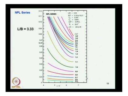
So, that is the high speed resistance so based on the test carried on based on these particular shown for the models, they have systematic did their model test and the resistance or results are presented in a in a systematic way. Here also, they used R R residual resistance by W, so against the displacement delta power 1 missing here. So, it will be delta power 1 length of displacement ratio and it is plotted for different fluid
