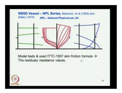
Next series is that is a round build semi displacement vessel is a NPL series, it is a national physical lab which stands for NPL, and it is in UK. So, they have a test specially it is they carried out systematic model test using the high speed this type of vessel and which comes under the NPL series under the results are presented accordingly, so here also ITTC skin formula is used.
