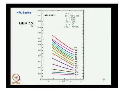
Similarly, you have the same thing L by B is equal to 7.5 here, so you have the values here so what you do is if your vessel is falling in between this. Suppose, you say here its 5.4 and here this is 7.5 suppose a L by B for the vessel which you consider is 6.5 what you do is you find out this value R R from here. That is for 7.5 due to this one you find out for this value then you interpolate the values, then you get the value for the 6.5.
