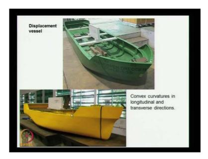
We can see that it is the shape you can see the transverse is convex and also you say longitudinal also, it is a convex shape. So, you can say that this is a displacement vessel which is having a convex curvature in the longitudinal and transverse directions. So, the convex curvature in the longitudinal and transverse directions, this reduces a flow separation at the stern and bilges. So, a smooth curve a convex curvature reduces that flow separation because it is a smooth shape.
