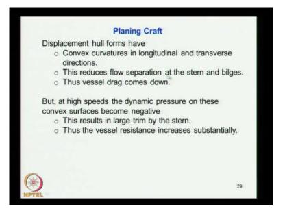
So, that is why it says there, it can be dynamic negative pressure mainly in the aft region, so what happens this results in the larger trim that is the pressure at the aft region gets reduced substantially due to the higher flow velocity. The subsequent reduced to pressure the vessel will trim more, thus the vessel when they trims more the hydro dynamic or the hydro performs the ship changes and the vessel resistance increases substantially.
