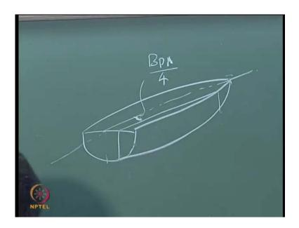
So, that is the B P A by 4 buttock line, so you look to what is the type of curvature you are getting at that point at that plan buttock plan. Then shape of a chine in plan what is the shape in the plan view and then shape of the sections all these are various parameters which will influence or affect the performance of the plan inverse, so this is the one what I said.
