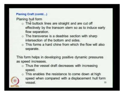
So, that is what the planning hull form buttock lines are straight and are cut off effectively by the transom. So, you if you find out that the buttock lines mean it is the longitudinal plain parallel to the longitudinal central line plain. So, if you curve a plane taken along the ship the longitudinal direction what I suggest is you consider a ship.
