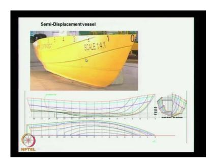
Then, you can see the spray raise here which you know, restrict the spray or arrest the spray and reflect the spray, so this is the form of a semi displacement vessel.
