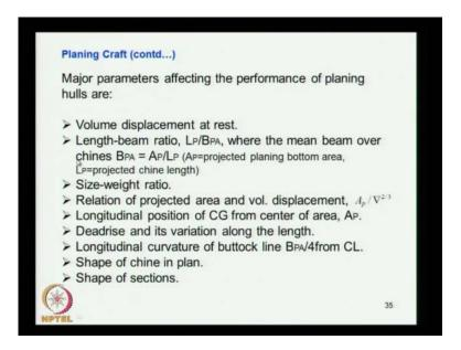
So, that is the one which diagram indicates major parameters affecting performance of planning hulls are volume displacement at rest. So, what is the displacement at rest which indicates whether the ship will generate sufficient hydro dynamic lift at higher speed? So, you can usually see that planning crafts are not big ones they are usually small to moderate, so the size is not so big length beam ratio that is L P by B P A, L P is a projected chain length.
