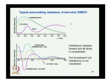
Similarly, instead of mono, you are now using what same as what you have seen, so this is a variation you can see the variation of the resistance co efficient forwards that twin struts. So, you have forwards and half strut, so you can see forward at a half strut what is the resistance radiation and of the hulls. We just sum it up you get the total resistance and here the same thing you can see that interference effects what is shown here interactions between strut and hull.
