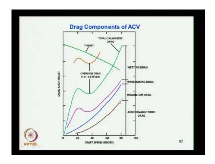
Drag components of the air cushion vehicle, you can see that drag component this is aero dynamic profiled drag. This is the momentum drag, then this is a wave making drag and this is a weighting drag that is the friction. So, the total thing you put you get the total drag and you know the thrust is the self propulsion point.
