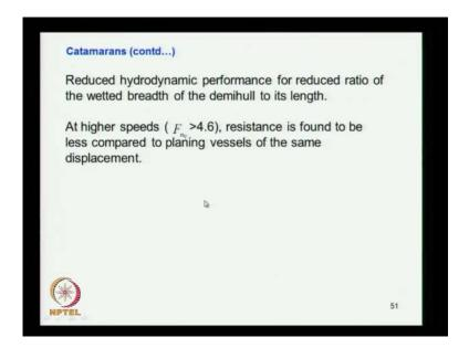
The reduced hydrodynamic performance for reduced ratio is of the wetted breadth of the demy hull to its length. So, it is related to wetted breadth that is underwater maximum breadth to its length, so the hydrodynamic performance should be reduced for this ratio is plus at higher speeds that is volume fluid number.
