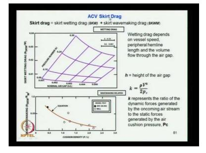
You can see the skirt, so I am not going to the details that can see the figure here this is a skirt weighting drag what is given here and this is skirt wave making drag. You can find from this this parameters values, here it is plotted against P by L P by L is I think pressure by length H by L, H is the air gap that is the chamber height divided by length of the cushion.
