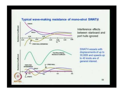
Swath is instead of two struts what you have seen here you have few using two struts, so mono strut means this is a joint together to have single strut. So, that is the mono strut, so you consider a vessel with a mono strut, then you can see the resistance given here resistance co efficient of the swath given separately. This is of the hull separately and then the difference affects separately, so from which you will get the total resistance of the vessel for different fluid number.
