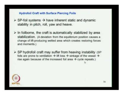
Surface piercing foils system have inherent static and dynamic stability, so they are stable all the hydro dynamic features of that have been inclined to one side. Automatically, the side which goes down will get more lift it will push it back it get generate some moment. So, its inherent automatic stabilization, so it will have in pitch role yaw and heave in foil borne, the craft is automatically stabilized by area stabilization.
