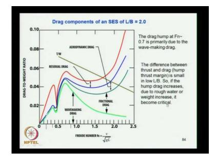
You can see this is a characteristic variation of different components wave making how its varying friction and then you have the residual drag then hydro dynamic drag. So, all put together you get the resultant one. That red line here that is the total drag to weight ratio for the surface effect of the ship having length to breadth of air cushion is equal to 2. (Refer Slide Time: 41:32)
