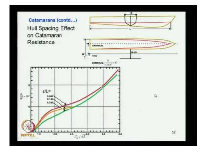
So, if you properly design and place it, then the resistance will be not greater in even Catamarans, you can see that these are resistance, you can see R T by W. It is displacement into 10 square that is what is total area and you can see this is for different s by L spacing, there is decimal spacing. So, if the spacing is less, interference effect will be more and resistance will be more if the spacing is more between the hulls interference effect will be less.
