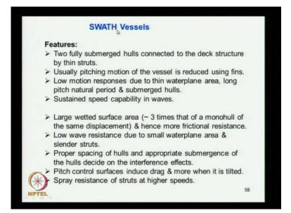
So, here the features of swath I think you understand what the swath, so I am not going give a definition sketch view of that. So, here the swath vessel the features two fully submerged hulls connected to the deck may be I will there is a diagram.
