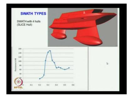
We consider the another one called four hulls, one here, two hulls here and another two hulls are this side four hulls is again the swath, you can see the variation of the resistance like it speaks up some point.
