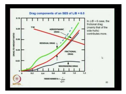
So, the resistance and thrust match here for the components, you can surface of the ship which follows L by B is equal to 6, you can see the fluid number and here its drag to weight ratio R by W, you can see that what is the wave making drag is very less, you can
