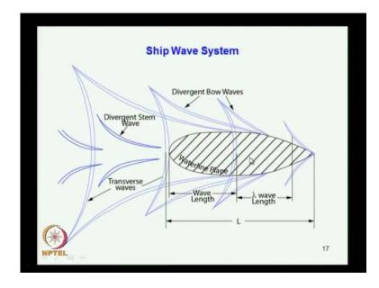
This is another systematic representation of that ship base system, we can see the ship waves are generated and the give this a divergence wave is coming out. And these waves which tangentially you know join at you know, which get such a shape converse shape here this is called the transverse waves. And these waves systems are generated from different regions of the ship, you can say that starting from here another system from here another from here another wave system from here.
