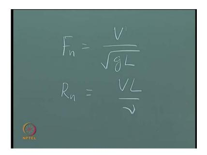
V L by mu is a Reynolds expression, where V is the flow velocity L is the characteristic length dimension of the body and mu is the kinematic viscosity of the fluid. So, if you consider the bow part of the ship alone, the bow part is having a small length. So, V L by mu L is a small length speed remains same if you can consider mu also remains same. So, that means the local Reynolds number is less, so low Reynolds number naturally will have laminar flow.
