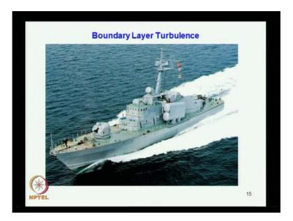
Similarly, you can see the boundary layer turbulence of a vessel you see the forward side is very almost smooth flow, and when it comes towards the way from the forward we say that it becomes foaming. Hence you always note that the foam region represents the turbulence, in the flow. So, the forward region you can say the local length is small Reynolds number is less and the flow is laminar. So, when it goes towards raft the length increases Reynolds number increases, flow become turbulence.
