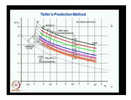
One of the method is put forward by Telfer and is known after him as Telfer's prediction method. We can see here, the graph shows total resistance coefficient usually is put as 10 cube c t because of the value of numerical values it is quite small. Usually it is better to plot you know 10 cube c t and against the Reynolds number here. So, here in the Telfer's method, it tries to satisfy a Reynolds number and a Froude number from the model test.
