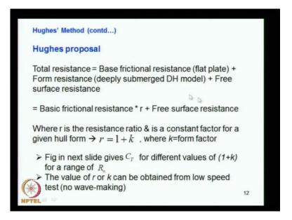
So Hughes what do I put here is the total resistance is now constituted by the base frictional resistance at the flat plate which we have seen, using the previous formula plus the form resistance deeply submerged double hull model. So, double hull model is the one which I have discussed before. So, it is a deep form resistance plus free surface resistance, that is the wave-making resistance.
