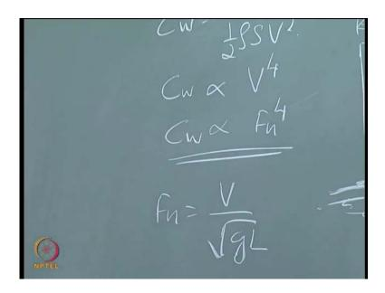
So, that means C w is proportional to C w is proportional to now V power 4 or we know that Froude number is equal to V by root g L. So, we can say that this is now proportional to Froude number is to 4. So, C w is proportional to Froude number raised to 4. So, that is how we have written like that C w is y, y is a constant into Froude number raised to C w is proportional to Froude number raised to 4. So, y is a coefficient and F n is the Froude number.
