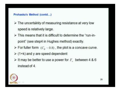
So, the uncertainty of measuring the resistance at very low speed is a relatively large. So, when you measure the resistance is very low at very small Froude number, very low speed. So, measurement become also becomes difficult when you use a small quantity. This means that it is difficult to determine the run in point that is you have seen the Hughes method what is the run-in point that is the slope which comes during the bottom.
