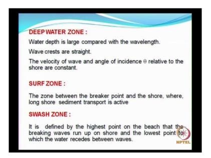
So, these are the important zonation of the waves and this is what is shown in this slide. As I have already explained all these things surf zone, swash zone, of course breaker zone is defined by just one line that is the zone of wave breaking.
