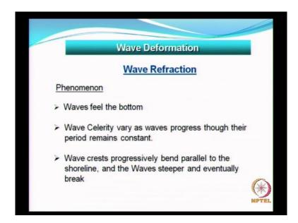
So, let us look at wave refraction. Waves feel the bottom; that is what I said. Waves feel the sea bed, presence of the sea bed. The speed of the wave varies as waves propagate through their period, remaining although their period is going to remain constant. Wave crests progressively bend parallel to the shore line and the waves steepen and eventually break.
