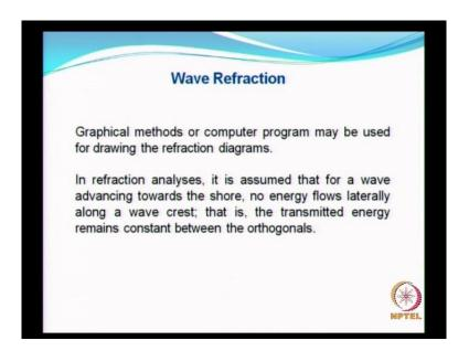
As I said the earlier, graphical methods or computer programs may be used for drawing the refraction diagrams and all other the points also have been discussed. No energy flows laterally along the wave crest; that is, the transmitted energy remains constant between the orthogonals. All these points are extremely important.
