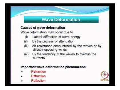
What is meant by wave deformation? Any kind of deformation of the wave surface, we call it as wave deformation. What are the main causes for the wave to deform? Although there are several causes, the most important causes for the wave deformation to take place are the lateral diffraction of wave energy. What is meant by lateral diffraction of wave energy?
