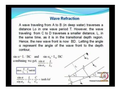
So, as a wave travels, we now consider a wave crest which is entirely in deep water and we also consider a wave crest which is a part of the wave in deeper water and part is in transitional waters or intermediate waters. When you take two wave crests in deeper water, so these are the two wave crests, this one and this one; the distance is separated by I naught
