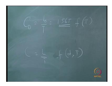
So, try to recollect deep water celerity is I naught by t which is just 1.56 into only a function of tau. It is not a function of water depth which we have already seen. The same thing only wherein shallow water, it will be I by t and it will be function of water depth and t.
