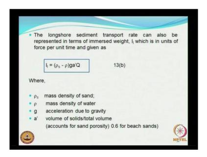
So when I do that, I can get an expression for the immersed weight; the immersed weight of the sand can be obtained as the difference in the densities; one is rho is the mass density of the sand, rho is the density of water and a dash is the volumes of solid divided by total volume which actually accounts for the sand porosity which in general it is set to be around 0.6 in the case of beach size. So, you see that there are a lot of approximations here and it depends on site.
