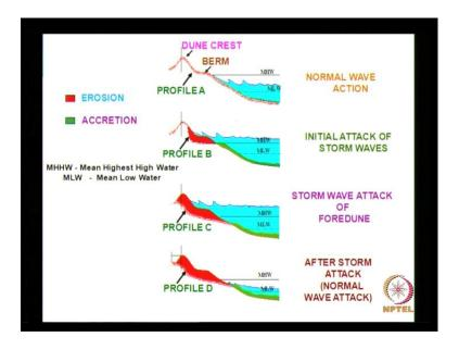
So, now we see the problem. In order to go in for the coastal protection, etcetera, we, first we will try to understand how this erosion takes place, coastal erosion, how it takes place? So, under this I will try to explain this phenomenon with the help of this slide, particularly when there is a storm that attacks a coast.
