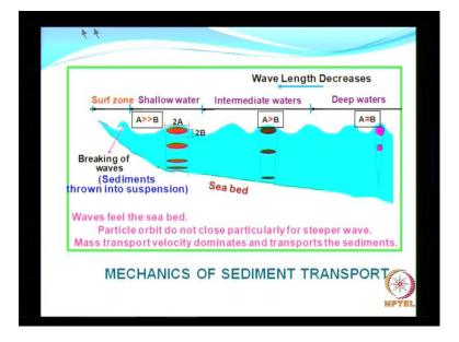
What does that say? That says, in deeper waters you have no effect of the surface waves on the sea bed. So, that means, the sand in the sea bed under this location will be more or less stable. But once the waves leave the deep water situation, once it enters intermediate depth condition, you know, it starts filling the bottom and the horizontal displacement will slowly reduce as it goes towards the sea bed, but still the affects of wave will be felt on the sea bed.
