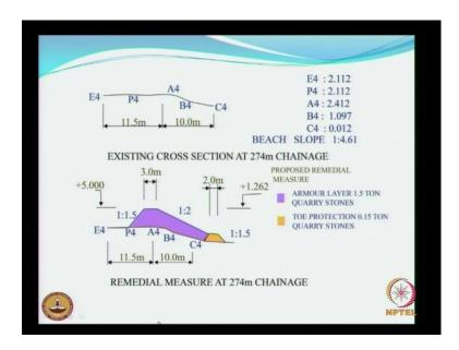
We have to look into the problem of what was happening. So, the sea wall that was in existence at certain stretches, we suggested as an immediate step, provide an armour layer of 1.5 tons of quarry stones and as toe protection, you see the toe protection is very important and this is the kind of temporary relief, so that, they can quickly get started with the rehabilitation of the sea wall.
