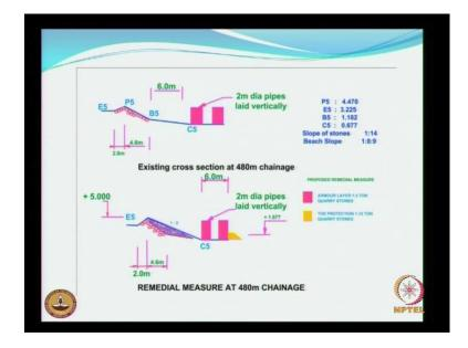
At locations where the pipelines were in vertical, these pipes, wherever they are vertical, they were vertical, we can easily see a lot of scour taking place. In fact, scour hole was there. So, what we had suggested is to protect the pipeline, because, removing the pipeline is going to be very expensive. So, you leave the pipe line as it is, but then protect it and then, but that was never done. So, some of those pipelines stood for some time and then collapsed.
