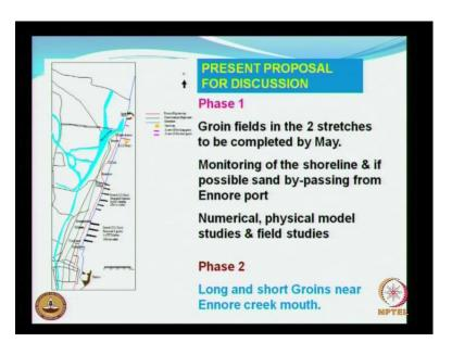
So, what we did is, the proposal after the survey, the initial proposal, this is the Chennai harbor and this is the Ennore satellite port. So, this is the first stretch. This is the two stretches. So, this is one stretch and this is another stretch. Groin field in the two stretches to be completed by May. We will come back to the groin field later. Monitoring
