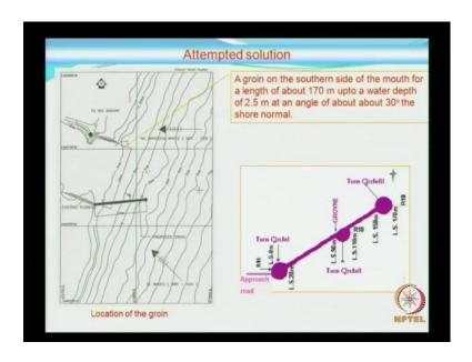
So, a groin on the southern side of the mouth of length of about 170 meters up to a depth of about 2.5 at an angle of about 30 degrees was subjected, was proposed. As you can see here you see those still because this these are supposed to be this is for the vehicle which carries the boulders to turn nothing else and these is not...
