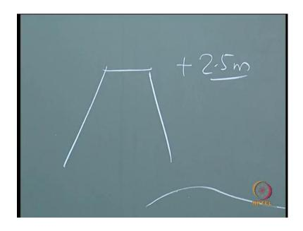
For such a groin the top level is also very important, here the top level was adopted as plus 2.5 meters plus 2.5 meters.
