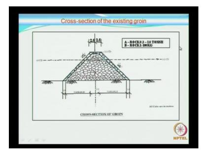
So, you look at the cross section that was adopted the cross section was one ton, and then inside the core layer inside the core layer it was around a it it was around 100 kg.
