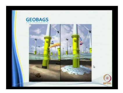
This is a application of geo bags of shore wind plants wind energy plants which is gaining a tremendous importance these days. So, when you operate when you go in for wind form, this is one important area where we need lot of information, scour protection forms a basic necessity.
