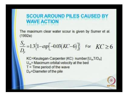
Scour under piles caused by wave action this basically a function of Keulegan-carpenter number, Keulegan-carpenter number is U max T by D. So, this equation is a quite straight forward, but it is valid only for K C number greater than 6.
