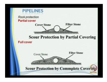
Then this is in case of a pipeline, this is only a partial protection you have you protect only for this portion. Probably in deeper waters, because if this kind of a situation exists in shallower waters, the ship anchors etcetera might hit by chance.
