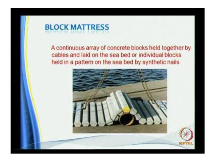
So, this is another block mattress a continuous array of concrete blocks held together by cable and then it is a laid over the concrete block; see for example, you look at this is to take care of end scour.
