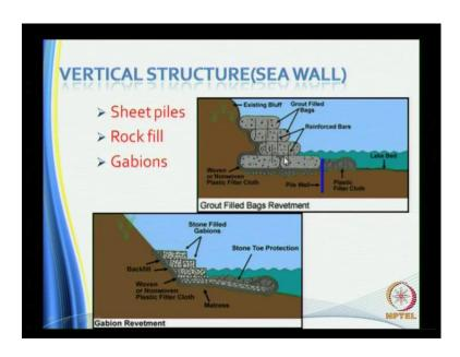
So, this is vertical walled structures sea walls as I have told you these are used by using gabion's. See scour and erosion they are together infant there is a slight difference, but the effect is almost same effect is loss of material.
