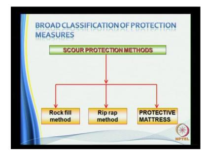
Broad classification of protection measures the scour protections methods can broadly be classified as rock fill method, riprap method and protective mattress.
