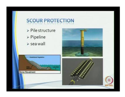
So, you see that there is a pile structure here how a how it has been protected you see that this is the kind of protection. So, the width a height all these things need to be calculated or you can have a stone revetment in order to provide, prevent this slope erosion the scour around this. And you can also have a vegetation here, which is strongly recommended, this is for the case of a pipeline you have a kind of a mattress.
