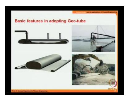
The basic features of in adopting a geo tube. This is the geo tube the length maybe as I said up to about may be 10 meters, 20 meters or 30 meters. So, you keep filling. You may have 2 or 3 holes also, pumping points wherein you pump the sand and then slowly the tube gets elongated and after sometime once you have done it full extent, it will form as as I said a solid unit and hence it can be retained. So, here you see a geo tube being filled in presence of water.
