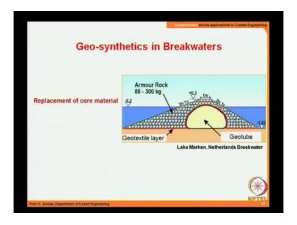
The same thing what I have shown you earlier, when you are dealing with this kind of a geo tube with stone on top make sure that you have run make sure that you run a geotextile over this. So, you see that red color that is the geo textile layer.
