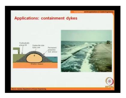
This is the coast and this is serving as a kind of a sea wall and you have here, it can be containment dy dykes wherein you can have the geo textile tube as the core and then over it you have to, you can have the stones. This is only for saving the material, but then from aesthetic point of view you are not really solving that problem because still it is going to be stones when you go in for this kind of a a design.
