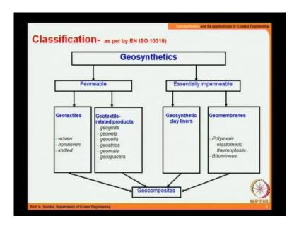
A broader classification of geosynthetics are as you can see here you can have either permeable or essentially impermeable. Under permeable you have further two classified products one is geotextiles, geotextiles mostly it is just a sheet or geotextile related products as you can see here, you have under permeable you have geotextiles and geotextile related products. Whereas, under essentially impermeable you, we have geosynthetic clay liners and geo membranes.
