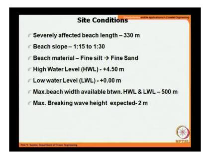
The site conditions are severely affected over a beach length of about 350 meters, the beach slope was measured to be ranging between 1 is to 15 to 1 is to 30, beach material consists of fine silt and fine sane sand, high water line is plus 4.5 meters, low water line is 00, maximum beach width available between high tide and the low tide, high water line
