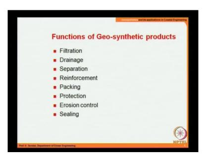
Functions of geosynthetic products. We have several role or functions of these geosynthetic products. One is filtration, then drainage, separation, reinforcement, packing, protection, erosion control which is the most important aspect or the function in the field of coastal engineering and then finally, sealing. So, you see a variety of functions of geosynthetic products.
