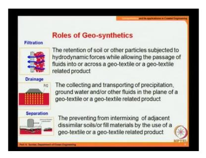
Now, this is further explained here concerning the, I mean the role of geosynthetics. The filtration as you can see here, the retention of soil or other particles subjected to
