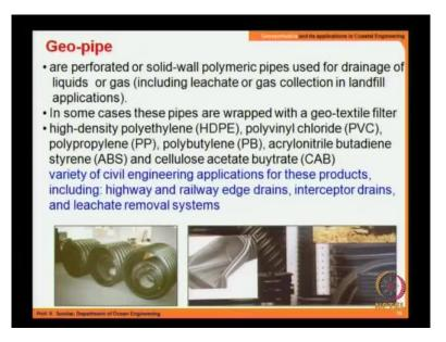
Next, geopipes, geopipes are perforated, it can be perforated or solid pipes of poly polymeric pipes used for draining liquids or gases including the leachate or gas collection in land fill applications. In some cases these pipes are also wrapped. So, you have a pipe, it is also wrapped over a geotextile. High density HDPE or PVC or PP or PB are some of the products material that is being used for manufacturing these geopipes.
