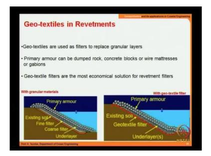
So, let us move into geo textiles, application of geo textiles in revetment. These are used as filters to replace granular layers, primary armour can be dumped, can be dumped rock or concrete blocks or wire, wire mattress or gabions. So, this is how it looks like. You have the geo textile running through the red color, over it we have the under layer or the filter
