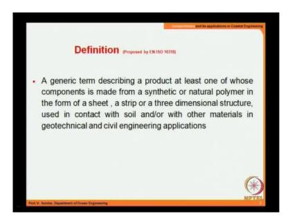
Let me start with the definition. This definition clarifies in brief what exactly is geosynthetics. The, a generic term describing a product at least one of whose components is made of made from synthetic or natural polymer in the form of a sheet, a strip or threedimensional structure used in contact with soil and or with other materials in the field of geotechnical engineering or for that matter any other field of civil engineering.
