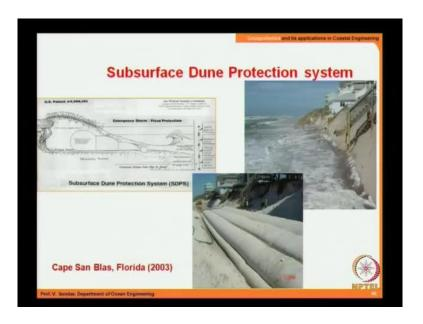
Then these are all subsurface dune protection. So, you look at the geo tubes here. You can just go into the Google and then try to look into look into the details, all the complete details are available. So, here you see that a number of geo tubes are formed in order to have a a protection like this. So, what could be planned also is have geo tubes as you have seen.
