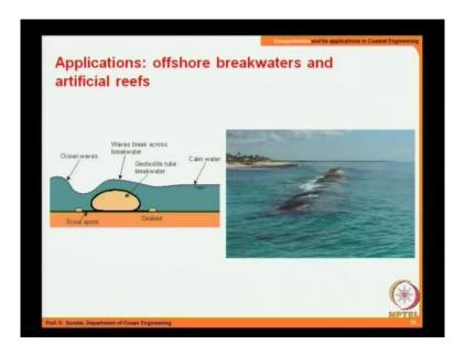
So, artificial reefs or offshore break waters. Offshore break waters we have already seen, offshore detached break waters can serve as coastal protection measure. That is one application, then artificial reefs. What is meant by artificial reefs? This artificial reefs can be submerged at a distance certain distance from the shore line. So, these artificial reefs will enhance pre mature breaking thereby you can have a a beach in front of in between the shore line and the artificial reef.
