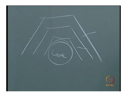
So, instead of core layer, so core layer, as you would recollect, you have the armour, secondary, core. So, this is replaced with the geobags.
