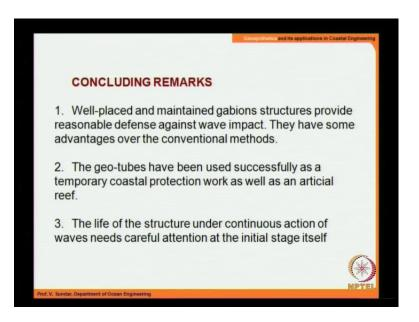
So, concluding remarks, well-placed and maintained gabions structures provide reasonable defense against wave impact. They have sometimes some advantages over the conventional methods. The geo-tubes have been used successfully as a temporary coastal protection work as well as artificial reef. The life of the structure under continuous action needs careful attention at the initial from the right from the initial stage itself.
