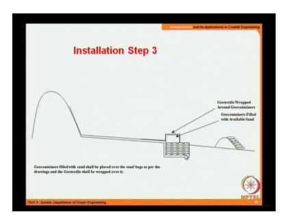
Then, you have the geotex, geocontainers filled with available sand. These are slightly bigger than the geobags and now this is how the toe was constructed.
