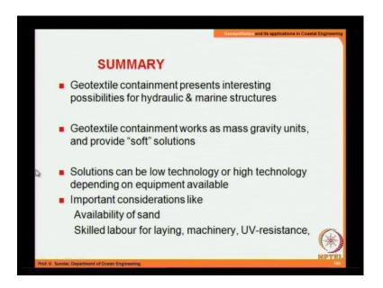
And so to conclude this, my lecture on geosynthetics, geotextile containment present interesting possibilities for hydraulic and marine structures. Geosynthetic containments works as mass, mass of the gravity unit and provide real soft solutions.
