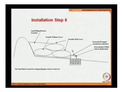
And you have the geotube fill, filled up and geotube with the UV resistance cover. Once this is done, the sand filling between the geotubes was done.
