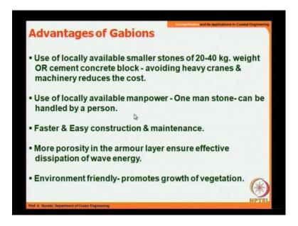
Advantages of gabions, use of locally available smaller stones of, maybe, up to about 40 or even 50 kgs or cement concrete block sometimes they will use. So, you avoid heavy cranes and then machinery. And then use of locally available manpower, one man can
