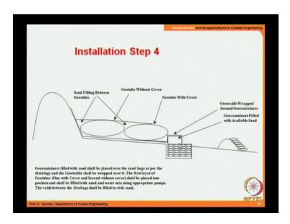
Once this was constructed, then the two geotubes are placed over this geotextile and then after this the third one is also placed.
