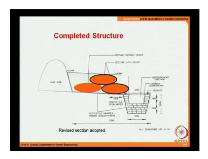
And this is, finally you have this kind of a cross-section that was implemented in Shankarpur. Once this was done what happened was, this was done initially for about distance of 100 meters and surprisingly we saw, that the geotubes were intact, but kind of a tilt took place because of yielding of the toe. This is a kind of an exposed toe, kind of a toe. Although I used the word excavation, but the depth of excavation is not much, so that means, it can be still called as.
