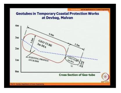
So, the idea was to have geo-tubes as shown here, one 3 meters diameter Geotube and 1 meter tube and this one, 1 meter dia geo-tube is to just act as a toe.
