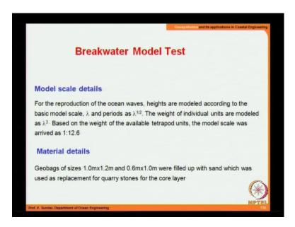
For the production, reproduction of the ocean waves, heights are modeled with a model scale of lambda and the period will be alpha, I mean, lambda into square root of lambda and the weights will be modeled as lambda cube. This I have already mentioned during in the lecture on stability of breakwaters and based on whatever units we have, that tetrapods. So, we had used it as 1 is to 12.6.
