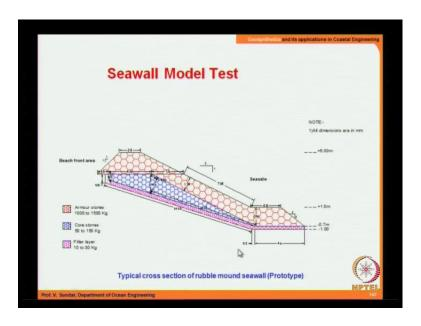
So, this is in, so the case of gabions. So, what we have done is, seawall, as you see here, are all this things, are core stones. This is core stone and this is a filter layer and this is a armour stone, as you can see here. And the armour stone is 1 tonne to 1.5 tonnes and instead of having this portion and this portion, has been replaced with gabions.
