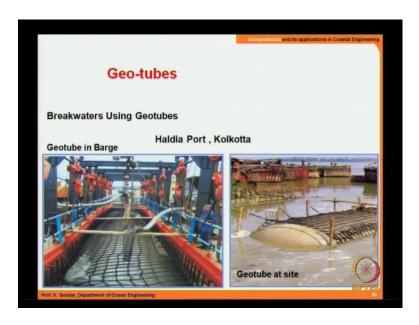
So, it is for, so that is application of a geotube. You see, the geotube is taken in a barge and then geotube is laid at site. This is mainly to protect the caving in of the site, slopes of a approach channel. This is somewhere in Haldia port and this was very successful project so far.
