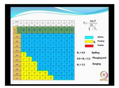
So, the parameter which we had defined earlier is N 1, and N 1 is the ratio of the beach slope and the square root of the wave steepness. So if you look at this table, what we have done here is, we have assumed the deep water wave height as 1 to 10 meters in intervals of one meter, and we have assumed the beach slope here tan beta in orange color. As you can see here from 0.01 to 0.1 in steps of 0.1, 0.01, and then here the green color the values
