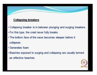
So they have examined while doing so, they have also found out another type of breakers and this collapsing breaker is found to be in between plunging and surging breakers. For this type, the crest never fully breaks. So the crust will be more or less looking stable. The bottom face of the wave becomes steeper that is the bottom portion of the wave becomes steeper and that is before it really collapses, and when it collapse it generates lot of foam.
