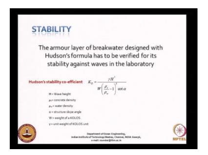
So, now, let us look into the how these make use of this some of these models or facilities for testing the break water stability. So, the stability of the breakwater as you know this controlled by the Hudson's formula has to be verified in the lab. So, these things I have already explained earlier, now there is we have seen DOLOS.
