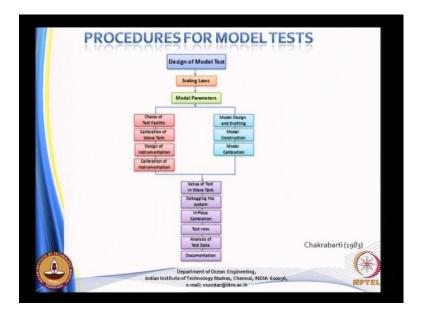
Procedures for model test; so you have to design the model test then apply a scale law, then you have to select the model parameters then choice of the test facility has to be chosen. Then calibration of the wave tank, calibration design of instrumentation, calibration of instrumentation. So, all these things are extremely important then you look at one is the test facility and other one is the model design and drafting model construction model calibration.
