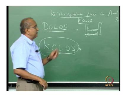
So, what we have done is we have recently introduced a name called KOLOS what happened was this DOLOS which was used you had I am not, so good in drawing. You heard 3 legs this leg was quite long, because of which there was lot of shear failure. So, the performance wise as an interlocking, and other aspects this was good, DOLOS was good, but individual unit it was having a problem.
