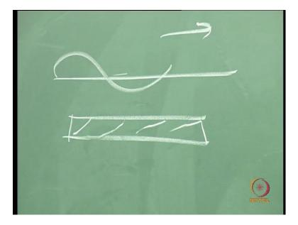
So, when you have flow taking place a waves moving in this direction and then in the wave flume you want to have submerged breakwaters plate breakwater for example, just an example. So, without the submerged breakwater you can look at the orbital velocities, for a given particular wave condition.
