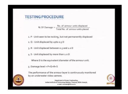
So, testing procedures percentage of damage is number of units displaced by total number of units. So, when you place the no total number of units are known to you the total numbers of units is known to you, then number of units displaced that you need to measure either you do it physically going and standing near the section or you can have camera mounted in the control room both facilities, we have both we both methods we adopts.
