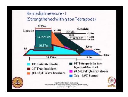
So, we continued the idea was to have an extra layer of tetrapod as shown here 9 ton tetra pods in two layers, and this was suggested with a strong toe for these 3 meters.
