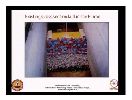
So, what we did was we just modeled this structure that is this is the existing structure. So, we have modeled here and this blue and blue and red co color they indicate one is 18 ton and another has 12 ton.
