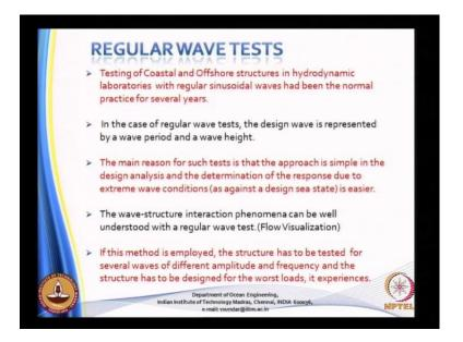
Now, regular wave test, testing of regular testing of coastal and offshore structures in hydrodynamic laboratory with regular sinusoidal waves has been a normal practice for several years. So, it is very, very simple because you have a tank, you have some mechanism where in the wave maker can be moving up and down like this or you can be moving in this direction.
