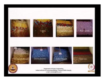
What we have done earlier is on cubes, cubes, Tetrapods trunk, Accropods, Tetrapods head section, DOLOS trunk sections, DOLOS head sections, Core loc. Then KOLOS also we have done and there are some many other models which I have not shown here.
