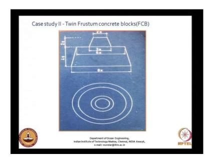
Next study again on stability test is shown here. Here there was a request to investigate the stability of twin frustum concrete block, and we were requested to look into its possibility for probably using it as one of the harmer unit artificial harmer unit for costal structure may be a breakwater or a seawall or whatever it is.
