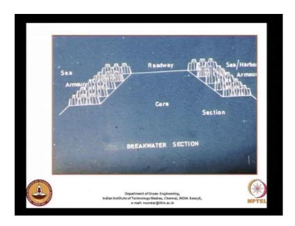
So, I do not want to go in to all the details but then I want to just show you what happened in this. So, there is no way to examine this through numerical model; you need to resort to physical model studies. So, this is the schematic representation of this. So, you have the core and over which it was thought that we can have a two layer of two layer or single layer whatever it is of these blocks.
