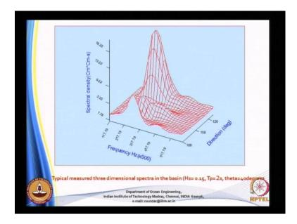
So, this is how a spectral density looks like when you have the three dimensional waves being recorded. So, you have the distribution of energy versus spectral density that will be the 2d spectrum but when you show it as a function of direction, then it becomes a three dimensional spectrum. So, for each direction you will have a spectral density or for a given frequency you can have a directional spread; any doubts in this, so that completes.
