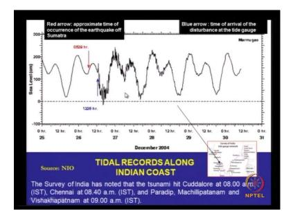
So, even Mormugao did not record at the time of failure because probably this failed your it failed to record the level slightly more than, what it is supposed to record.
