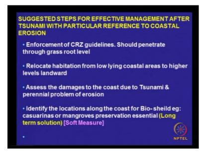
So, suggested steps suggested steps for the effective management after tsunami with particular reference to coastal erosion, enforcement of CRZ guidelines. CRZ guidelines is nothing but the coastal regulation zone so this there are some guidelines, which we have to adhere to should penetrate through the grass root level. So, everyone should know what is CRZ, so relocate habitation from low lying coastal areas to high level higher level landward.
