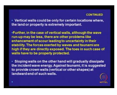
Vertical walls should be constructed only at locations where, the land or property is extremely important further, in case of vertical walls, although the wave run up may be less, there are problems like enhancement scour, leading to uncertainty in it's stability. The forces exerted by waves and tsunami are high, if they are directly exposed to then the toes toes of such structures has to be properly protect, has to be properly designed and executed.
