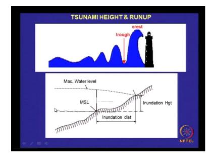
So, this shows that, this is the MSL elevation that is, mean sea level, when the maximum water level comes usually, it may be somewhere here. Mean maximum water height mean sorry maximum high water line may be somewhere here, may be may be somewhere here its only approximate representation. But during a tsunami, the maximum water level can may be much higher which means that it will run, it will reach the land point somewhere here.
