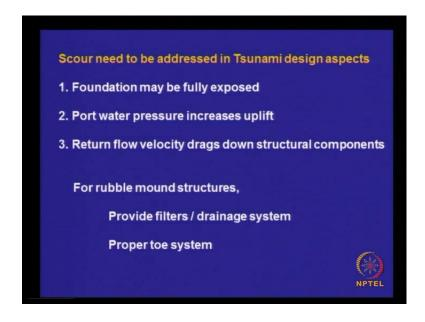
Scour need to be addressed in tsunami design aspects, foundation may be fully exposed, pore water pressure can increases increases up uplift, that is another problem. Return flow velocity drags down structural components, these are the effects due to the scour taking place. For mound rubble mound structures, you may need to provide a filters, drainage systems and proper toe systems.
