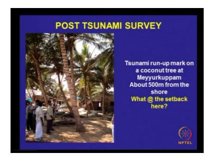
So, we did the tsunami run up mark see for example, we identified the coconut tree in one of the places and about 500 meters from the shore, what is the set back here. So, I will come back to the set back line later because how close the people can put up the dwelling units from the coast, this is one important issue, which needs to be discussed.
