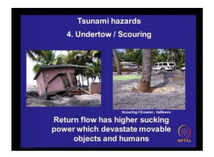
Then the tsunami under toe and scouring as you can see here look at the devastation effect of this building. The whole thing is toppled and you see the retaining water makes
