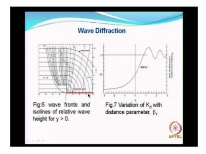
So, you can obtain the value of the diffraction coefficient. You, I will show you the next figure. You have a rigid breakwater here, and this figure shows the wave fronts and the
