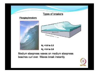
Then comes the plunging type of breakers, and I am sure that, you would have seen a number of advertisements also, wherein you have plunging breakers. It looks very nice. And, when does this occur, when medium steep waves on medium steepness, steep beaches and the waves curl around, and the breaking is instantaneous; wave instantly breaks and it also creates sound, when it breaks.
