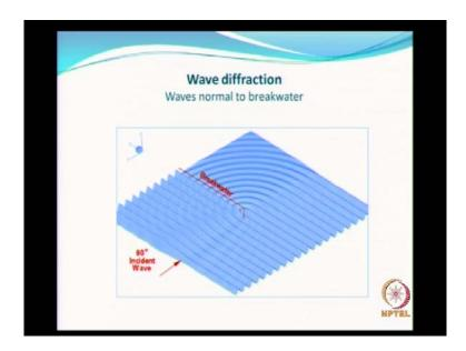
So, this is an animation, wherein you see the breakwater here, the presence of breakwater. The waves are moving, and after it is impinging on the structure, you see that, this moves uninterrupted; this is what I was explaining earlier. And, you look at the diffraction. And naturally here, the wave climate is expected to be very, very less; and, you look at this area, you see that, you have the reflection taking place. So, this animation itself shows us the phenomena of diffraction very clearly.
