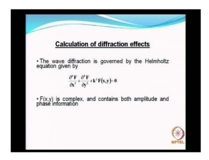
So, diffraction calculation is not so easy, compared to what we have seen earlier, in the case of, compared to refraction. So, wave diffraction is governed by what is called as the Helmholtz equation, where this F of x y, x y is in the horizontal plane, is a complex and contains both amplitude and phase information.
