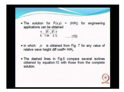
So, the solution to F of x y which is nothing, but directly the relationship between, the ratio between the wave height inside the sheltered area to the incident wave height, can be obtained as given here, x by L, L is nothing, x and y are the spatial coordinates and the beta r is, can be obtained in the next figure, that is next slide, which I, which, you have to see figure 7 in the next slide.
