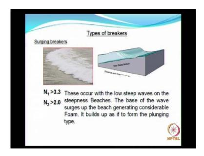
Then, surging type of breakers. This occurs with lower steep waves, on very steep beaches and the base of the wave, the base of the wave tries to surge up the beach, as if it is going to, generating considerable amount of foam, as if it is going to form as a, a plunging type of breaker.
