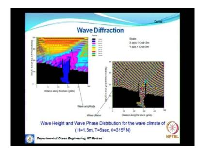
So, here, earlier we saw normal wave angle, angle of incidence. Now, we have the...So, this is called as phase contours, wherein this shows, how the waves try to move; and, you look at this, you see that, the waves are bending and waves are bending and then, once it enters a narrow area, it becomes complicated, because you have reflection from the sides, breakwaters, etcetera and so, you will have a different issue.
