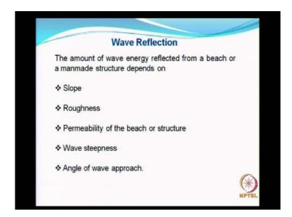
So, this, I have already explained; once again, let us see this. The amount of wave energy reflected from a beach, or a manmade structure, depends on the beach slope, the roughness, permeability of the beach, or the structure, wave steepness, as well as the angle of wave approach.
