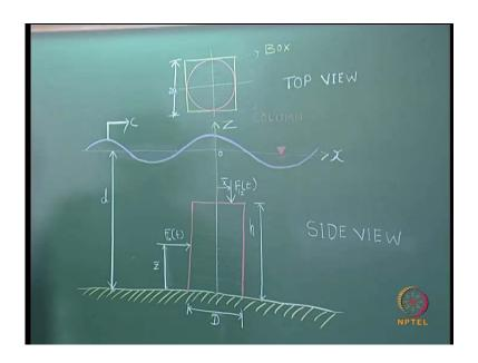
So, we are considering two surfaces, this is surface one. And the horizontal force is going to act in this direction over this surface. And the vertical force is going to act over this surface. And the respective centre of pressure, we are assuming to at a distance of z bar from seabed and from the central axis at a distance of x, the vertical force will be acting.
