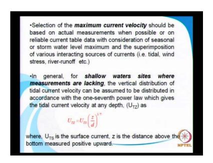
And now, how do you select the maximum current velocity? This should be to actual measurements, when possible or on reliable current table data. And we need to consider the seasonal or storm level maximum, and superposition of various interacting sources of current. For example, you have the tide induced current or the due to very often, the most although, we have some of these river-runoff, wind stress etcetera. The tide induced is going to be quite dominant.
