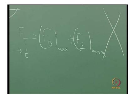
Can we add directly maximum drag force and maximum inertia force, to get the total force? Can I say that total force equal to F D max plus F I max? It is not correct. Because when you look at the values, you are going to be overestimating the forces.
