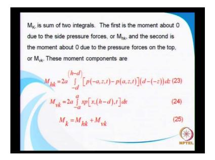
So, you have to now, for example, (No audio from: 12:24 to 12:30) in a similar way you need to get the expression for the force in the vertical direction. So, now straightaway I am just using these expressions, for the moment due to the horizontal force and the moment due to the vertical force that is what is given here.
