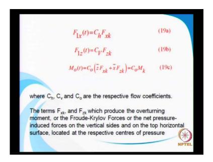
Here, as per the Froude-Krylov force, the horizontal force given by equation 19 a will be a product of some kind of a flow coefficient, which may be determined or given to you by through experimental published literature through experimental investigations. And that will be equal to f into f suffix k x of k. And similarly, the vertical force is given as shown here. The moments or cost by these two forces, at point o which is at this location.
