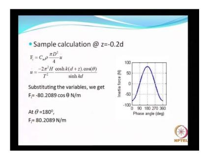
So, I am just showing you, a sample calculation by taking z equal to minus 0.2 water depth.
