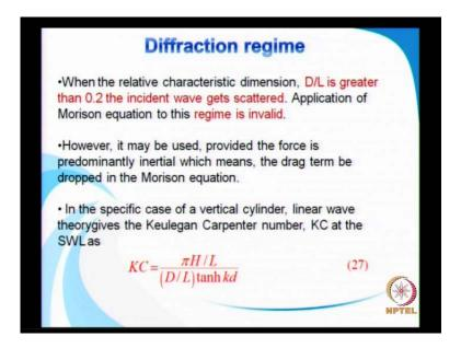
Now, with this, what I will do is, I will, we will come back to the wave forces, but prior to doing the taking up the diffraction regime. We will just look at the some of the problems, through which we can understand the wave forces. I have taken a pile to illustrate, the effect of different parameters on the wave forces. That is the intension of this lecture, one is to demonstrate the calculation process.
