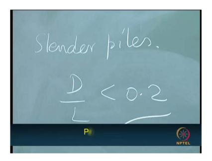
We have earlier seen the wave loads acting on slender bodies. So as we talk, as we have seen earlier, when we talk about the structures, we normally talk about slender piles first, slender piles when D by L is less than 0.2; where in, we had used the Morison equation or the equation proposed by morisonetal in 1950. And, that is well entrance in literature, there is absolutely no ambiguity in using it, but although there are some certain uncertainties which I have already discussed.
