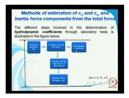
I means the linear theory, and then you can determine the hydrodynamic coefficients as I have just mentioned, this is one of the methods, but there are other methods to determine C d and C m. So, this is from the force, and from the from the measured elevation you obtained the U U dot, etcetera from the measured force. You you correlate these three to get the hydrodynamic coefficients; that is what this is explained in this slide.
