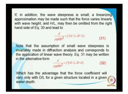
And then, that will boil down to three parameters. In addition, if we are considering that wave steepness is small then, linearizing approximation may be may success the force will vary linearly with wave height.
