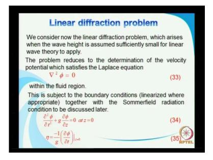
So, now let us look into only the basic things. So we consider, the linear diffraction theory which arises when, the wave height is assumed to be sufficiently small. So that is, we are basically, we are we say that the linear theory is applicable.
