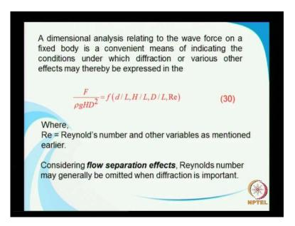
So the purpose of dimensional analysis you should be knowing. So mean, there are several problems where you can solve forces on structures using numerical model.
