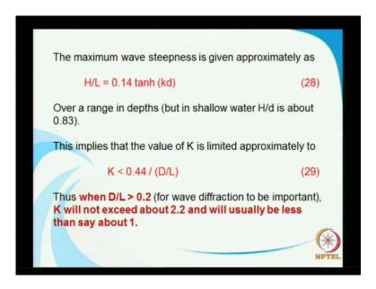
Some of these are basic information's are necessary. The maximum wave steepness is given by that expression 0.147 into tan h kd and then over a range in depth but in shallow waters the H by D about 0.83. This implies that, the K is limited approximately to that expression given in 29 equation 29.
