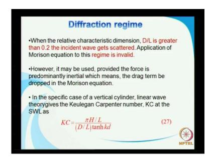
So, this is normally said to be in the diffraction regime, and if you look at slide here; so when the relative characteristic dimension D by L is greater than 0.2, the instant wave after striking the subject object it get scattered.
