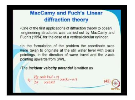
So I will just present this method which is analt analytical solution and its quite straight forward in order to obtain the values or the forces on large bodies, in the formulation of the problem the coordination access originate at the still water as per our usual definition then the instant velocity potential is taken as cosine, in this case we have taken as cosine you please refer to our wave mechanics equations, I think probably we would have considered sin theta for velocity potential.
