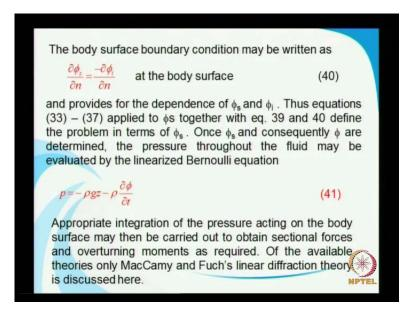
So, the body surface boundary condition can also be written at a body surface as a mentioned in equation 40. Now this 40 equation now, this is going give you the dependence of the scattered potential.
