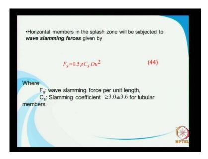
So, we have an empirical relationship to get that we slamming force and the horizontal members particularly in the splash zone will be subjected to such slamming forces and that is given to given as a similar to what we have seen the drag force so you have a slamming force here that is the only thing which is not known, and slamming provision can be approximate said to be equal to 3 to 3 and a half 3.6 for tubular numbers.
