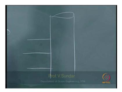
So, for the so initial integrate get the force acting over a particular section. Like that, you do you do force entire structure and then integrate, you will get the total force acting on the pile, so we are talking only about a pile here.
