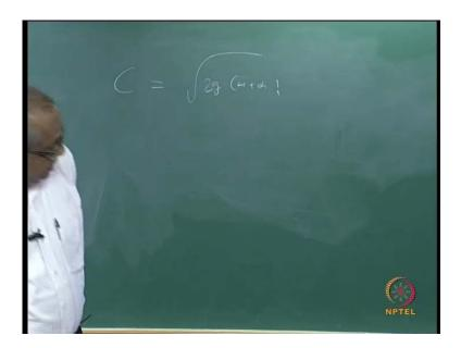
In this case, the celerity the speed of a solitary wave is given as root of, which we will see later. The profile given by, represented by the solitary wave can be represented as shown here, this is sec and H. And here, all other parameters known to you X is being the origin at the crest, based on this only, you can draw the profile, is that clear? A different values for a given C, given characteristics of H, and d use these expressions and
