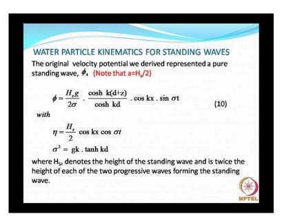
Now, let us look at the water particle kinematics for standing waves (No audio from 26:08 to 26:29). The original velocity potential may be phi 3 of the form of either phi 3 or phi 4, it does not matter, you can take anything which ever you want. So, the original form of a velocity potential that in this case should be phi 4, what we have derived is for a pure standing wave.
