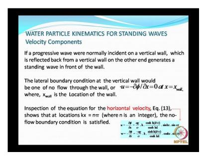
Now, again we continue the particle velocities, particularly when we talk about a vertical wall, when we have a vertical wall, what is the first, what is that kinematic bottom boundary condition, vertical velocity normal to the sea bed is 0, now you are having a vertical wall and you have a wave coming and hitting the wall.
