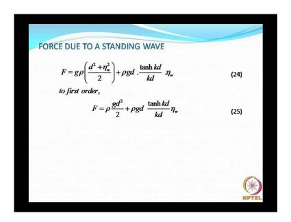
So, once you do this, the first order wave force due to a standing wave can be directly obtained and as you can see here. So, this can usually be used for calculating the wave forces on a vertical wave. However, you can cap with the pressures at the different elevations along the wall and integrate it.
