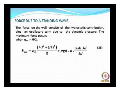
The force are consists of hydrostatic components as well as the dynamic component. So, what I will do is, anyway this completes the basics of the standing waves up, and when we are talking about the wave forces acting on vertical walls that that is coastal structures
