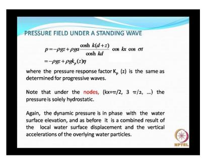
So, this is continuous and there is what you would have and note that, under nodes under nodes that is equal to k x equal to pi by 2 or 3 pi by 2, etcetera, you see that the pressure is going to be solely hydro static is that clear. So, after the lecture, you please have a look at the slides, go through carefully, slowly, I am sure that you are in a position to understand.
