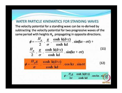
So, particle kinematics in the case for the standing waves, the velocity potential for a standing wave can be re derived re derived by subtracting the velocity potential of two progressive waves, herein we are considering two progressive waves, but when will the standing wave take place, when they are moving in the opposite direction when they are moving in the opposite directions.
