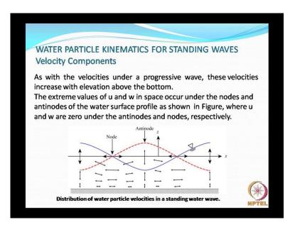
Now, as the velocity under a progressive waves as with the velocities increase with the elevation, the particle velocities are kinematics is going to with respect to the variation along the depth, it is similar what is going to happen when a progressive wave passes.
