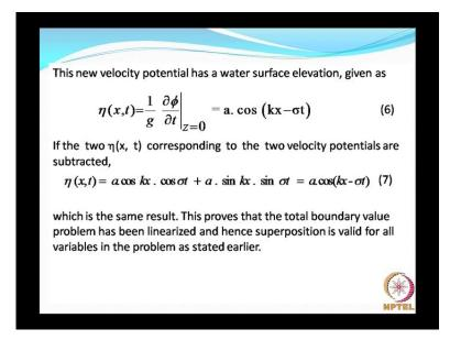
Now, this velocity potential is bound to have the eta variation as shown in here, that is it is going to be for a cosine curve. At this point of time, I would like to reiterate what I have said earlier.
