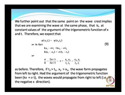
Or we further point out that the same point on the wave crest implies that, we are examining the waves with the same phase.
