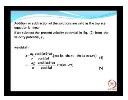
Strictly speaking, we are subtracting phi 3 from phi 4 phi 3 from phi 4. When we do that, the resulting equation will be as shown in equation 5, this is nothing but our classical velocity potential which we have already seen.
