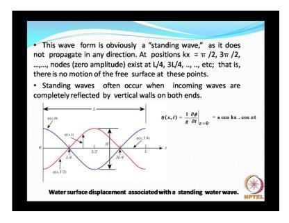
And that is what it is illustrated in the right hand, in the figure in the right hand corner below. Now, this form is obviously a standing wave, because it does not propagate, it is not propagating.
