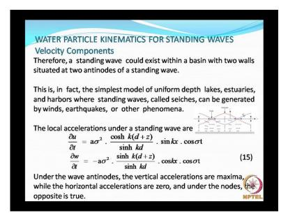
Therefore, a standing wave could exist within a basin, for example we have a wave basin or we have a vertical wall I mean a flume, now you remove the wave absorber, you generate a wave, allow the wave to, allow the wave maker to run for some time, what will happen, the wave will travel, go hit the wall and come back, and what will happen you will initially have some standing wave for certain location, certain stretch.
