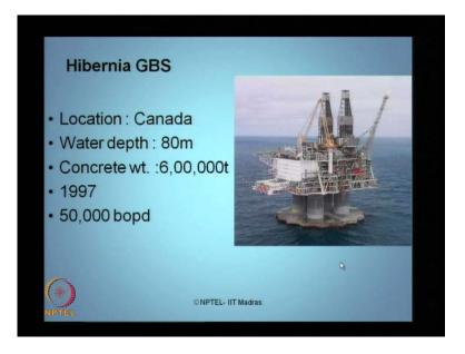
Hibernia gravity based structure is another example located in Canada at a depth of 80 meters. It is a concrete platform, the concrete weight alone is above 6 into 10 power 5 tons, some massive construction systems build in 1997, produced about 50,000 BOPD.
