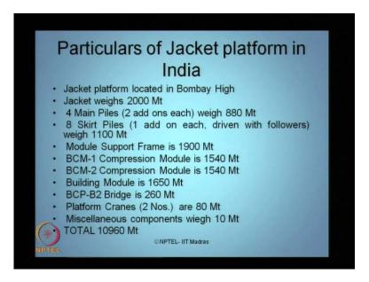
We also have jacket platform constructed in India, in Bombay High. The jacket weighs about 2000 metric tons, resting on four main piles, 8 skirt piles, module support frame weighing about 1900 metric tons and the compression module one, two weighs about 1540 metric tons each. The building module weighs about 1650 metric tons constructing a total of weight of about 10960 metric tons in total.
