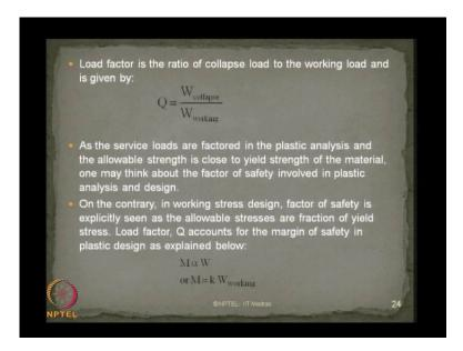
So, the load factor which an arbitrary value selected, which is the subject of interest is defined us the ratio of the collapse load to the working load, which is given by simple expression as you see on the screen now. As the service loads are factored in the plastic analysis and the allowable strength is close to yield strength of the material, one may
