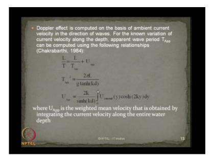
In the absence of the detailed effect of Doppler's effect on stretching of waves because of presence of current; Doppler Effect is computed on the basis of ambient current velocity in the direction of waves as you saw in the last slide. For the known variation of current velocity along the depth apparent wave period can be computed using analytical relationship is given by chakrabarthi in 1984.
