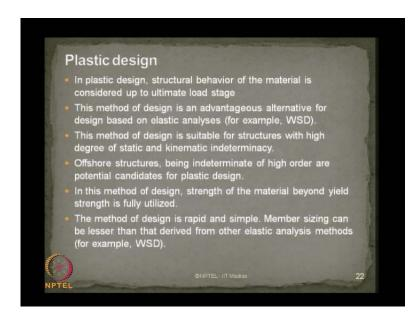
Once I get the allowable stress value can always design the member or I can get the permissible value get the dimension of the member which is otherwise called as design of the structural members of offshore structures. Now, alternatively in the recent pass the searches of started practicing what is called plastic design in offshore structure.
