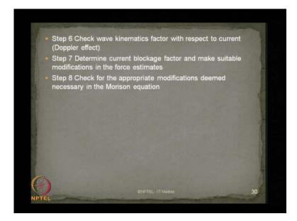
In step number 6, you check wave kinematics factor with respect to the current is called as Doppler's effect; in step number 7, determine the current blockage factor and make suitable modifications in the force estimates; in step number 8 check for the appropriate modifications deemed necessary for the Morison equation and ultimately design the members.
