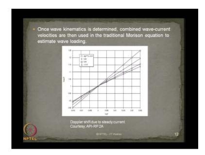
Ladies and gentlemen, in this figure shows what is the variation which can be having or it occurs from the Doppler shift due to steady current which is taken from API RP2A as a courtesy. So, once wave kinematics is determined combined wave current velocities are then used in the traditional Morison equation to estimate the wave loading.
