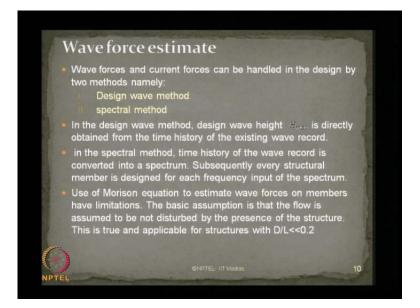
Once I have defined the form for a specific offshore structure, once I have chosen a site, once they are the oceanographic hydrographic data specific site, then I am interested to find out what are the wave forces coming on the members in the offshore structure design and located at the specific site. The wave forces and current forces generally handled in the design by two methods, namely design wave method and spectral method.
