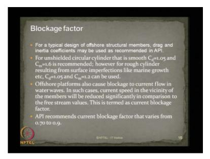
Now, what is the blockage factor? For a typical design of offshore structural members, drag and inertia coefficients are generally recommended from the American petroleum institute coral provisions for unshielded; for example, there is a circular cylinder which has got no members in near vicinity, we called this as unshielded circular member.
