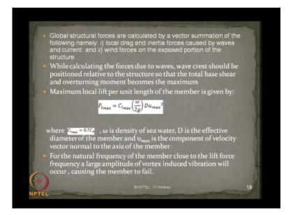
After knowing this, the global structural forces are then calculated by a vectorial summation of the following. One is compute local drag and inertia forces caused by waves and current in a segment; compute the wind forces on the exposed portion of the structure; while calculating the forces due to waves, wave crest should be positioned relative to the structure.
