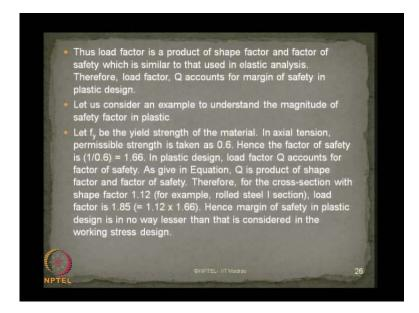
Thus the load factor is nothing, but the product of shape factor and factor of safety which is similar to that used in the elastic analysis. Therefore, a load factor Q which accounts for margin of safety in plastic design can be considered the margin of safety which is seen here in the other design factors.
