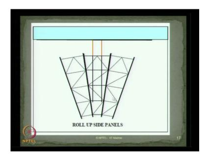
Once the side panels are ready then roll up the side panels to the proper required alignment as you see in this figure.
