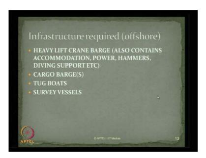
Adding to it, heavy life crane barges as you see in the previous slides, which also contains accommodation, power, hammers, diving support etcetera which are available on the crane barges should be made readily available during installation of jacket structures. You should also require cargo barges, tugboats, survey vessels etcetera of during installation of template structure.
