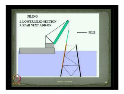
Then the second step will be lower the lead session and then add on into the next session. I am keep on loading the lead session and adding the sub sequence section to the lead section, so what we call as piling operation.
