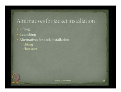
They are alternative arrangements are also available for jacket installation. Can either do lifting or launching; it can also do alternatives for deck installation as lifting or float over.
