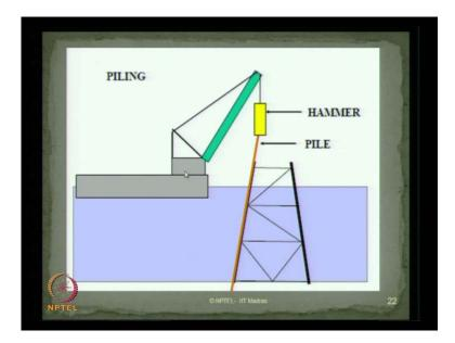
Once it is completed then you drive a hammer and starts driving a pile of this specific leg into the sea floor, using a special kind of crane barge, which has a capacity of pile driving.
