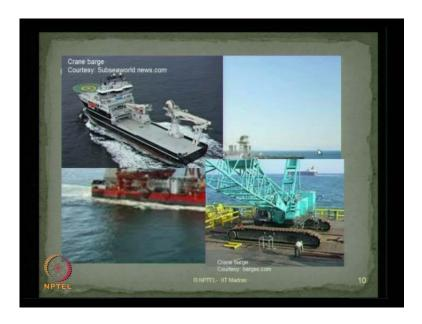
We can also have a crane barge whether barge can housed different specialization of crane, which can be also use for holding the jacket structure in position during driving. You can also have a crane barge with a special kind of equipments as you see in this photograph.
