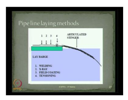
So, they are different process takes place in the laying of the pipe once you lay the pipe or once you keep the pipe on a barge which we call as a lay barge. Then I have to first do welding of barge then I have to check the welded joint using x-ray diffraction techniques then I will do apply field coating on the fabricated joins at the entire pipeline then I have applying tensioning system before it draft the pipeline using articulated stingers.
