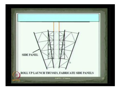
Then you roll up the launch trusses and fabricate this side panels. These are the launch trusses and now the figure shows the fabrication of the side panels.
