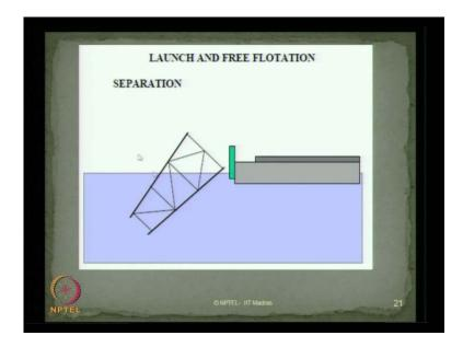
Once it is made to dive then the separation takes place and the jacket template gets away or gets this disconnected from a rocker arm of the barge, so this is what we call as separation.
