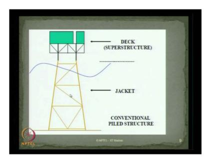
Now the sequence of figures what you see now will tell you the sequence of construction and installation procedure of a conventional piled structure. So, it is the deck which you see on the top side in green color which we call in the super structure this is supposed to be a mean sea level this is we call as a jacket. This is a photographs are schematic view of a conventional piled structure.
