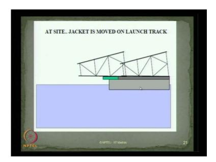
At site once, the jacket is moved on the launch track, now the barge is grab to the side and then subsequently the jacket is tip over what we call the rocker arm. Over a rocker arm the jacket is tipped down.
