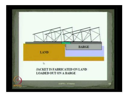
Now you have completed the fabrication and it is ready for load out. After fabrication is now complete, we will think about the steps about launching. So, you place it on a barge, because this is a land where you fabricated. These are the steps sequence of steps involved in moving the fabricated truss or the jacket template to the barge jacket. The jacket is now fabricated on land and load out on the barge the operation of shifting to the jacket barge is what we call as load out.
