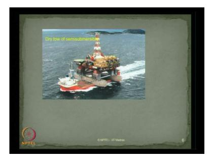
This photograph shows you the dry tow of the semisubmersible. So, this is the semisubmersible kept on a barge and being go to site for exploratory drilling. So, we call as dry tow operation of semisubmersible.
