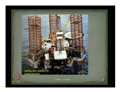
If you look at the construction or installation sequence in terms of jacket platforms, which was see in previous slides. The current slide shows you jack up with platform in a raised position. You can see here these are the jack up legs and this is the platform in a raised position.
