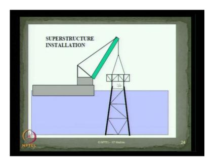
Then I am bringing the top deck, which is brief fabricated from the yard using a barge using a special kind of crane vessel, I lift this specific facility and do the connection of the facility to that of the jacket this is what we call as deck mating in the operation.
