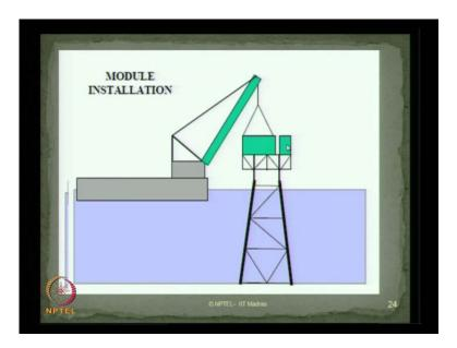
Once I completed the deck mating, I also keep on adding additional modules, which we call as module installation. This modules can we living quetzals, can have operational module, can have process modules etcetera are depending upon top side design of the
