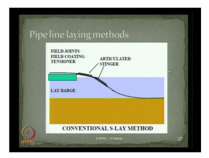
Alternatively, you can also use what we call s-lay method. The field joints, field coating and tensioner are all connected to the pipeline, and then the pipe is laid on a barge which we call as a lay barge. Then it is being articulated in a stinger and the pipe is laid as you see here. Since the profile of the pipe during laying forms a shape similar to S, we call this is S-LAY method of pipe laying.
