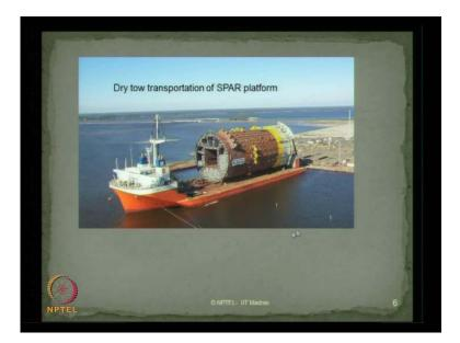
This is again a dry tow operation of a SPAR platform. This is actually a SPAR, which is being kept on a big barge, and therefore this operation is called dry tow. Ladies and gentlemen, it is easily recognize that when the body of the platform is not immersed in water then we call this as dry tow transportation. Alternatively, when you use the same vessel for transporting directly by the floatation principle then we call that as wet tow transportation.
