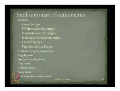
Let us quickly see the brief summary of equipments, which are generally used for offshore construction process. We can use barges like crane barges, offshore derrick barges, semisubmersible, jack-up barges launch barges and pipe line laying barges. Also offshore dredging equipments are used in case of in this kind of methodology, supply boats, anchor-handling boats, towboats, drilling vessels, and crew boats are some of the important summary of equipments are generally used for offshore project.
