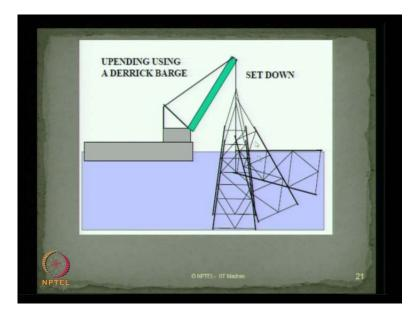
Once it starts free floating then I am going to use a special kind of crane or a semisubmersible for example, SAIPEM 700 which can do the upending operation.
