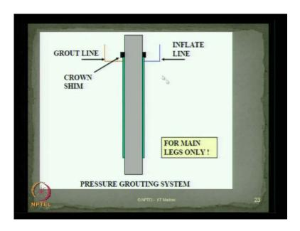
You can also have a different type of grouting system for the main legs of jacket what we call as pressure grouting system. In that case, I have a crown shim on the top and keep on doing a pressure grouting from an inflated line, what we call as a grout line keep on grouting from the grout line, and of course, keep on releasing the pressure from the inflated line as you see in the schematic view.
