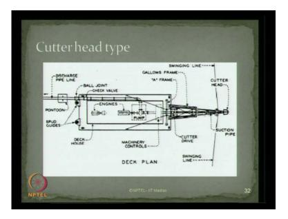
The figure, what you see here, shows the components and parts of the cutter type head
