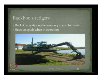
Backhoe dredgers have bucket capacity varying from 0.5 to 13 cubic meters. They rest on spuds when they are in operation. As you see in this picture here, these are the two different legs, what we call as spuds, in operation. This is actually a backhoe dredger, which is used close to the coastline or to river line for doing some dredging operation.
