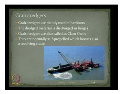
Grab dredgers are essentially used and commonly seen near harbours. The dredged material is discharged in barges, as you see in the photograph here. Grab dredgers are also otherwise called as clam shells. They are normally self-propelled, which houses also a revolving crane, as you see in the photograph.
