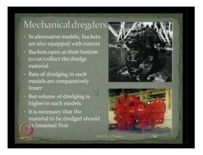
In alternate models, buckets are also equipped sometimes with cutters. The photograph, what you see here is bucket, which has got a cutter and a dredge. This is actually, typically, form of rotary cutter, which is used in form of the bucket to collect the sediments from the sea bottom. Buckets open at their bottom to collect or to cut the dredge material.
