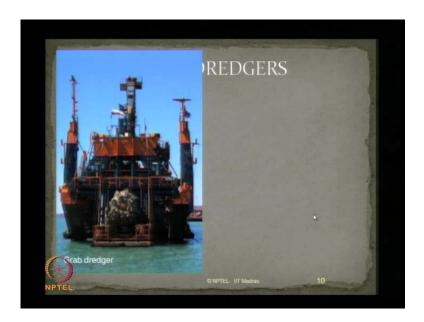
This is a grab dredger. As you saw in the previous lecture, grabs are nothing but buckets, which has got two half shells, which can open, then fix this spoil and get deposited in the containers.
