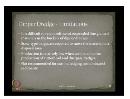
There are some limitations of this kind of dipper dredgers. It is very difficult to retain soft, semi suspended fine grained materials in the buckets of dipper dredges. Scow-type barges are required to move the material to a disposal area. Production is relatively low when compared to the production of cutter head and dustpan dredges; not recommended for using in dredging contaminated sediments.
