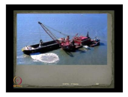
The photograph now shows you clearly, that this is clam shell bucket, which is doing dredging in this operation and keeps on transporting the dredged spoil into a barge. As we see here, this is actually a dredger, which is supplied with the self-propelled engine, which can be placed in position with that of spud cans.
