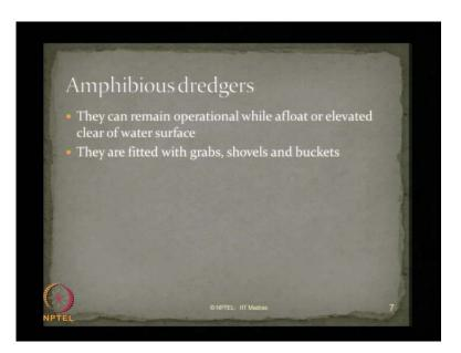
You also have amphibious dredgers. They remain operational while afloat or elevated clear of water surface. They are fitted with grabs, shovels and buckets, which are similar to that of mechanical type of dredgers, but of course in smaller size.
