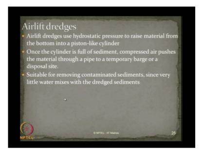
Airlift dredges use hydrostatic pressure to raise material from the bottom into a piston like cylinder. Once the cylinder is full of sediment, the compressed air pushes the material through a pipe to a temporary barge or a disposal site directly. Suitable for removing contaminated sediments, since very little water gets mixed up with the dredged sediments in this kind of operation.
