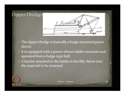
The other alternative mechanical type dredger, which we saw in the last lecture, is elaborated here. It is a dipper dredger, as you see, the dipper and shovel is provided along with this. These kinds of dredgers can also be position restrained using spuds. As you see in the figure here, the dipper dredger is basically a barge-mounted power shovel.
