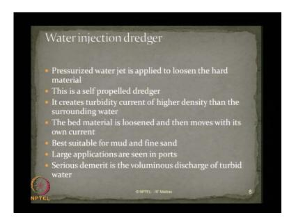
You also have water injection dredgers. The pressurized water jet is applied, essentially, to loosen the hard material, which is deposited this is a self-propelled dredger. It creates turbidity current of very high density than the surrounding water. The bed material is thus loosened and then moves with its own current into suction tube.
