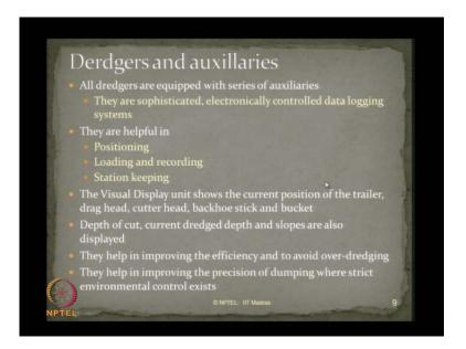
As you see, the dredgers and auxiliaries are also important. All dredgers are equipped with series of auxiliaries. They are sophisticated, electronically controlled data logging systems. They are helpful in positioning a dredger, loading and recording and station keeping.
