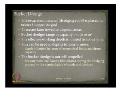
In case of bucket dredges, the excavated material, which we have addressed as dredging spoil, is placed in the scows, which is otherwise called as hopper barges. These are later towed to disposable areas. The bucket dredgers range in a different capacity, varying from 1 to 10 cubic meter. The effective working depth is limited to only about 30 meters.
