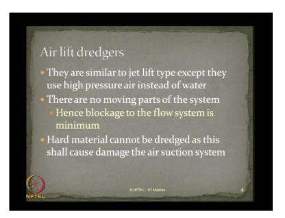
If you look at the air lift dredgers, alternatively, they are similar to jet type dredgers except that instead of high stream pressure water, these kinds of dredgers use high pressurized air. There are no moving parts in the system, therefore no blockage to the flow system and if at all any blockage occurs, that occurs to the minimum level of, on operation. Hard material cannot be dredged using this system, because this can cause damage to the air suction system in the dredgers.
