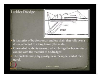
Ladder dredger is another type of dredger, which we saw in the previous lecture. I want to elaborate the parts of ladder dredger you can see here. Ladies and gentleman, this is ladder, which is having series of buckets. The fixed rate, the bottom of the bucket is what we called as the tumbler.
