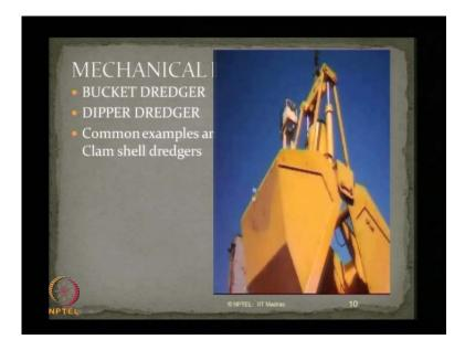
This is clam shell dredger, which you saw in a video in the last lecture how does it operate. Of course, these kinds of mechanical dredgers, though the operations has less volume of picking of dredge spoil, but the efficiency are much superior to a parallel bucket type or ladder type mechanical dredgers.
