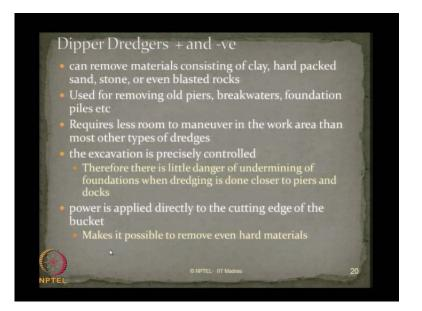
The merits and demerits of dipper dredgers are as follows. It can remove material consisting of clay, hard packed stone, sand or even blasted rocks from the spoil site. It is used for removing old piers, breakwaters, foundation piles, etcetera. It requires less room to maneuver in the work area than most other types of dredges.
