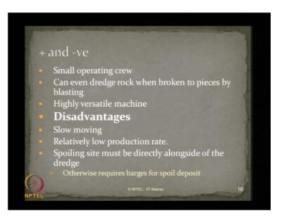
There are advantages and disadvantages of bucket dredgers. It requires only a very small operating crew. It can even dredge rocks when broken to pieces by blasting heavy versatile machine, which is very commonly used in harbors.
