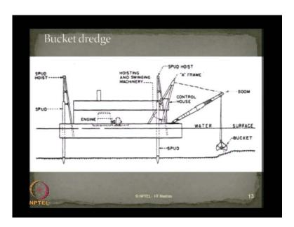
This is hoist and swinging machinery, which is actually used to operate the bucket for dredging operation. These are the spud hoist, which are controlling the movement of the spud veneration into the sea-bed when the dredger is under operation.
