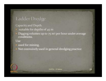
The capacity and depth depends on operational criteria of this kind of dredgers. It is seen, that this kind of dredgers are suitable up to depth of 45 meters. The digging volume varies from maximum 75 cubic meter per hour under average condition of operation. It can be used for mining, but not extensively.
