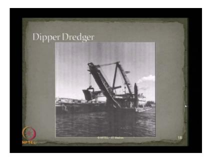
The dipper dredger operation is what you see in the photograph, here. This is a dipper; this is a frame, which you can see. The shape is A frame. The hoist, which is supporting the dipper, which has got a power shovel, which is forced into the material for dredging spoil and collected and then disposed of.
