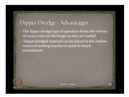
Salient advantages of this kind of dipper dredgers are, the dipper dredge type of operation limits the volume of excess water. That is very important because as the dipper fixed, the drains spoil from the side, water drains off during the operations itself. So, the volume of excess water in the barges, as they are loaded, can be minimized. The dipper dredge material can be placed in the shallow waters of eroding beaches to assist in beach nourishment parallelly.
