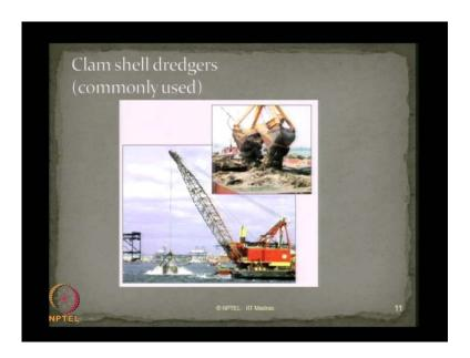
The commonly adapted clam shell dredgers, as pictures. As you see here, this is a clam shell, which has got two (()) in this center, which has cutting edge, as well as, this opens and dredged spoil is discharged. This is a photograph, which shows, that the clam is picking up the dredged spoil and supplied to the rotary crane, which can rotate and dispose this dredged spoil from the site to that of barge located nearby.
