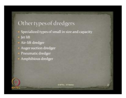
Other types of dredgers are essentially under the single umbrella classification of specialized types of small size and capacity and operational rate, they are jet lifts, air-lift dredgers, auger suction dredgers, pneumatic dredgers and amphibious dredgers.
