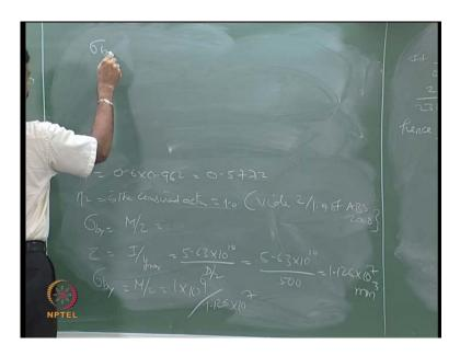
n 2 is for the combined action, which is taken as 1 in this specific case. This is as for clause 1.9 of ABS-2008. Sigma b y, in this equation, is simply M by Z. Let us compute Z as I by y max, in my case, which is going to be... So, sigma b y is M by Z, (( )) Newton meter by 1.126 10 power 7.
