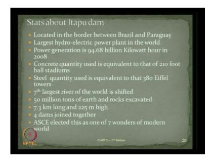
The Itapu dam is located in the border between Brazil and Paraguay. It is the largest hydro-electro project in the world power generation, is above 95, million, billion kilowatt hour in 2008. The concrete quantity used is equivalent to that of 210 football stadiums. The steel quantity used in this project is equivalent to about 380 similar Eiffel towers.
