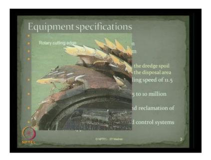
This is a closer view of the rotary cutting edge, which Aquarius uses for cutting and loosening of the dredged material.
