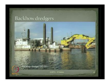
This is the picture showing you the backhoe dredger owned by Dredging Corporation of India, BH-1. This is the (( )), which lifts the dredge spoil. This is backhoe dredger hose from the vessel, which can be transported from one location to another location because it is self-propelled as well.
