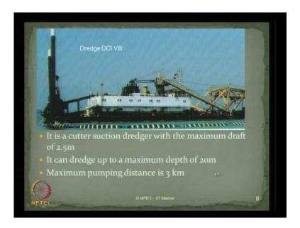
Dredging DCI-8 is the picture, which you see here, this is a cutter suction dredger with the maximum draft of about 2.5 meters, it can dredge up to a maximum depth of about 20 meters. The maximum pumping distance of the dredge spoil is about 3 kilometers.
