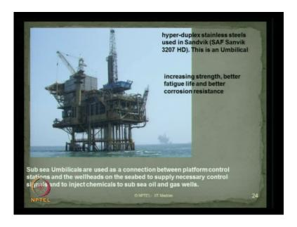
In this specific module, hyper-duplex stainless steel is being used in Sandvik, is an umbilical. Actually, this increase in strength, better fatigue life and better corrosion resistance has made the steel very useful for construction material. The subsea umbilicals
