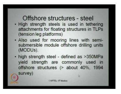
If you look down further high strength steels are used in tethering attachment for floating structures in TLPs, also used for mooring lines with semi-submersible in case of mobile offshore drilling units. High strength steel defined as yield strength more than three fifty mega Pascal are commonly used about 40 percent of offshore structural system use this as per survey shown in 1994.
