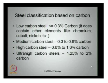
Now, if you look at steel classification based on carbon alone, you can further classify this as low carbon steel, medium carbon steel and high carbon steel. So, low carbon steel is the one which has got less than or equal to 0.3 percent carbon, it does not contain other elements like chromium, cobalt and nickel whereas, medium carbon steel as the percentage of carbon varying from 0.3 to 0.6 percent and high carbon steel has content varying from 0.6 to 1 percent of carbon.
