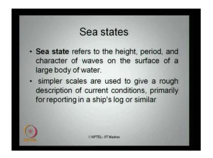
Let as look at different kinds of sea states for which the offshore structural system is subjected. Sea state refers to height, period, and character of waves on the surface of a large body of water. Essentially they are simple scales which are used to give a rough description of the current conditions, primarily for reporting a ship's log or similar.
