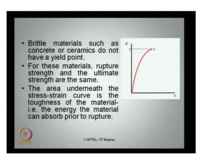
In case of the brittle material the story is slightly different; brittle material such as concrete, or ceramics do not have a designated yield point. In such cases rupture strength and ultimate strength are exactly the same for these members. The area underneath the stress- strain curve is an index of the toughness of the material. So, toughness is on the other hand energy of the material which can absorb prior to the rupturing of the material.
