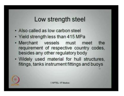
We can also classify steel further based on its strength as I said, low strength steel, medium strength and high strength steel. Now, let us quickly look at what do we understand by a low strength steel, it is also called as low carbon steel, yield strength is lesser than 415 mega pascal. The merchant vessels must meet these requirements of course, of different respective country codes, besides any other regulatory body.
