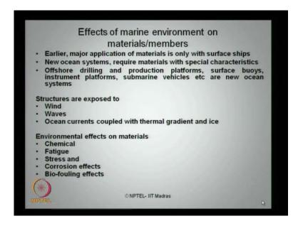
Now, let as quickly look at the effects of marine environment on members or materials used for ocean structures. Earlier the major application material is only surface ships, now the ocean systems require material with special characteristics. Offshore drilling and production platforms, surface buoys, instrumentation platforms, submarine vehicles, are new kinds of ocean systems which demand special characteristics material which can be used or applied on them.
