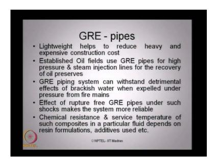
G R E pipes have light weight pipes and therefore, reduce the weight and the construction cost as well as, piping system is concern in offshore industry. They establish oil fields use G R E pipes for high pressure and steam injection lines for recovery systems. G R E piping system can be with stand detrimental effects of brackish water when expelled under pressure from fire mains.
