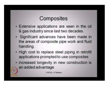
Extensive applications are seen in oil and gas industry in the recent paths in 50 years. Significant advantages and advance have been made in the areas of composite pipe work and fluid handling. High cost to replace steel piping in retrofitting them prompted people to use composites. Increase longevity a new construction is an added advantage which is gain by use of composites in construction material for marine applications.
