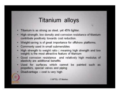
Titanium alloys are increasingly, commonly being used, now in offshore application. Titanium, ladies and gentlemen is has strong as steel, but yet about 50 percent lighter. High strength, low density and corrosion resistance of titanium alloys contribute positively towards the cost reduction and become attractive for this material to be recommended for marine applications. Weight saving is one of the important and great advantage, if we talk about design of offshore platforms.
