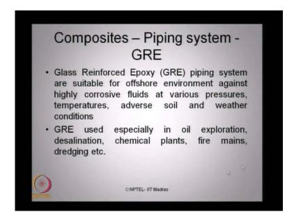
So, composites are recommended very fairly for piping system, as we saw in the previous guide. G R E is one of the important composite, which is glass rein force epoxy resin which it is a piping system which is suitable for offshore environment against highly corrosive fluid at various pressure, temperature, soil in weather conditions. G R E is popularly being used now, for oil exploration, desalination, chemical plants, fire mains, and dredging etcetera.
