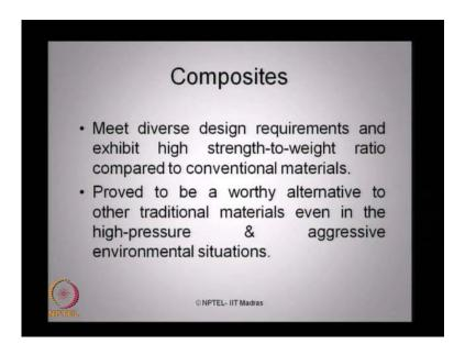
Composites actually meet diverse design requirements. They also exhibit high strength to weight ratio, that is at a lower weight material gives you higher strength. So, they meet highest strength to weight ratio compared with that of other conventional materials
