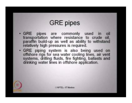
G R E pipes are very common, in all transportation as well, where resistance the crude oil, paraffin build up as well as ability with stand relatively high pressure are required as a important characteristic in case of transportation. G R E piping system is also being use on offshore rigs for sea water cooling lines, air vent systems, drilling fluids, fire fighting systems, ballast systems, drinking water lines in many other applications in offshore segment.
