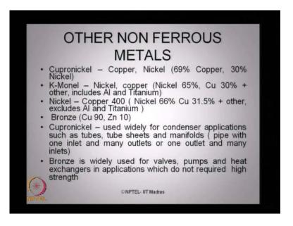
There are alternative non- ferrous materials like cupronickel, K Monel, nickel, bronze which are widely used for different upper tenancies lie valves, pumps, heat exchangers where no other material can substitute the strength and the functional requirements.
