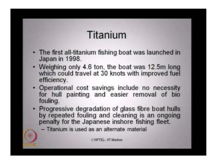
The first all titanium fishing boat was launched in Japan in the year 1998. Weighing only just 4.6 tons the boat was about 12.5 meter long which could travel at a phenomenal speed of 30 knots of course, there has been some mechanism diverge the fuel efficiency was improved in this boat to attain the speed. Operational cost savings include no necessity for hull painting and easier removal of bio fouling.
