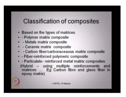
Based on the type of matrices, we can have a polymer matrix composite, metals matrix composite, ceramic matrix composite, and carbon fibre matrix composite and fibre rein force polymeric composite and particulate rein force metal matrix composites,. But cannot say have an hybrid variety as we discussed in the previous live.
