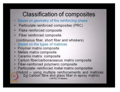
Let us quickly see, how composites are classified. Composites are essentially classified based on the geometry of the rein forcing phase. Particulate Reinforced Composites, which you call them as PRC. Flake Reinforced Composite FRC. Fibre Reinforced Composite (FRC). Continuous fibre, short fibre and whiskers can be again a sub classification in fibre, reinforced composites. It is also classified based on the type of matrices what we use.
