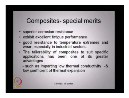
Composites are special merits, ladies and gentlemen, superior corrosion resistance, exhibition of excellent fatigue performance, good resistance to temperature extremes and where especially in industrial sectors, the tailor ability that is the constructability of composites to suit specific applications has been one of the major advantage of composites. Such as, imparting low thermal conductivity, low coefficient thermal expansion.
