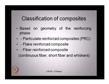
That is a very important advantage as phenolic gratings are concern. Let us quickly look at the classification of composites, based on geometry of rein forcing phase I can say particulate rein force composites, flake force composites, fibre forced composites, which is having continuous fibre short fibre and whiskers.
