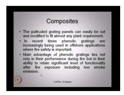
The pultruded grating panels can be easily cut; therefore, fabrication becomes simple and can be modified as per your dimension requirements. Therefore, fabrication construction easiness, dismantle and transportation, becomes as simple; so people get attracted towards the use of pultruded grating composites for top side construction in offshore industry. In recent times, phenolic gratings are also be extensively use in offshore application where fire safety has become important.
