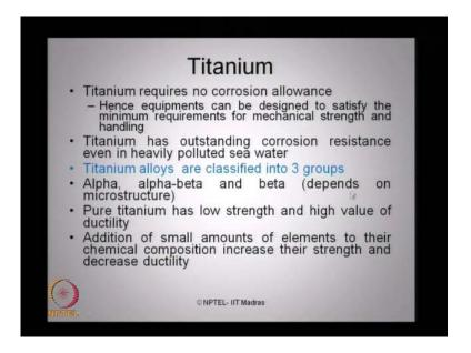
Titanium actually requires no corrosion allowance at all. Hence, equipments can be designed to satisfy the minimum requirements for mechanical strength and handling as well. Titanium is an outstanding corrosion resistance even in heavily polluted sea waters. Titanium alloys can be classified in to 3 groups, as you see, now alpha, beta and beta. This grouping of titanium alloys actually, depends on the microstructure of this material.
