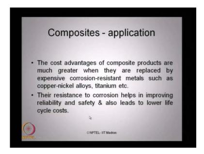
Composites also have many advantages and applications. The cost advantage of composite products are much greater when they are replaced by expensive corrosion resistant metals such as, copper nickel alloy, titanium et cetera. Their resistance to corrosion helps in improving reliability and safety and also lead to lower life cycle cost. It is a very important factor which is an important assessment in construction management technique of offshore industry.
