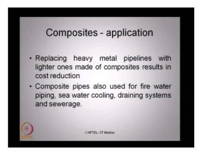
Composites, ladies and gentlemen, have now replaced heavy metal pipelines with lighter ones. Because, it is a phenomenal decrease in cost, composite pipes are also used for fire water piping, sea water cooling, drainage systems and sewerage applications.
