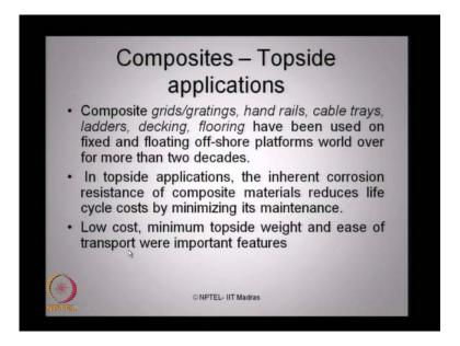
Composites also have very wide variety of applications in the top side. Composites grids, gratings, handle rails, cable trays, ladders, decks and flooring in offshore industry has become recently increasing, which have been used for fixed and floating offshore platforms world over. In top side application, the inherent corrosion resistance of composite material reduces, ladies and gentlemen the life cycling cost by minimizing its maintenance actually.
