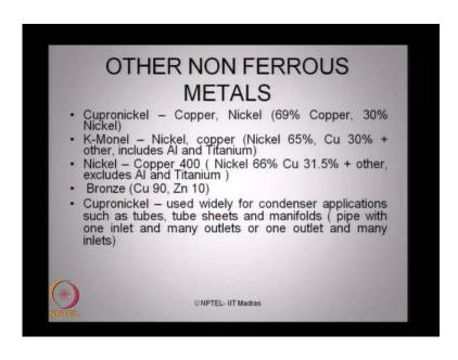
There are other non- ferrous materials which can be also used in offshore construction. For example, cupronickel alloy which is mixture of copper and nickel in the percentage of 69 and 30 is an alternative material for construction offshore industry. The other one which is very popular and being used is K Monel alloy, which is combination of nickel and copper at 65 30, and the other material like aluminium and titanium are also being included in fabricating a manufacturing this K Monel alloy.
