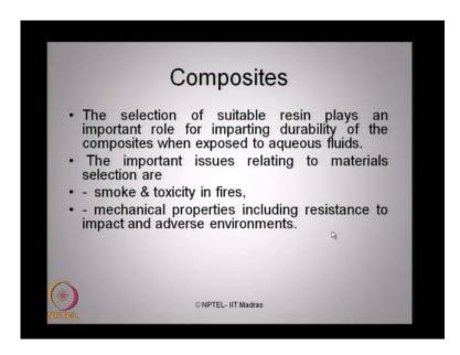
The selection of suitable resin plays a very important role for imparting the durability characteristics to composites when expose to aqueous fluids. The important issues
