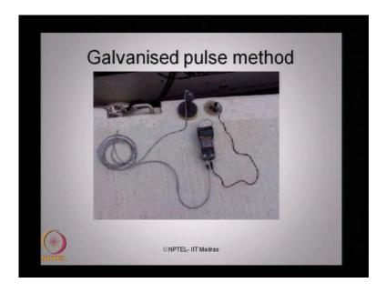
Galvanic pulse method is another technique, which can be used to identify the strength of concrete.
