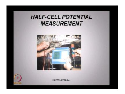
Half-cell potential measurement talks about the penetration of chlorides, which is responsible for corrosion of reinforcement.
