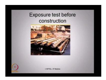
And of course, exposure test before construction is very practical method by which I tried to keep concrete members in the same environment as they will be subjected to in due course of time. Say very physical and practical method by which people will generally do these for adopting concrete in specific environment which they will be used
