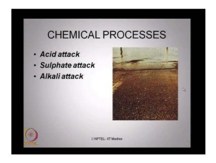
Chemical process can be resulting from acid attack, can be a sulfate attack, or can be a alkali attack, which forms a white component of white surface on the surface area of the concrete as well as parches which is having brownish and white component on the surface.
