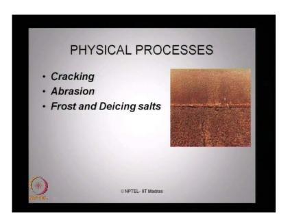
If you look at the physical processes much closer, the photograph shows you here is result of cracking, abrasion, frost and deicing salts, which are appear surface of concrete member as you see here.
