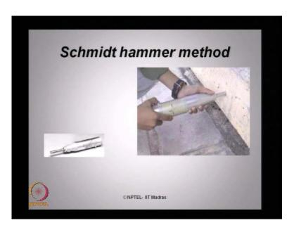
Schmidt hammer method, I am sure engineers would have heard about this, civil engineer and structure engineer are use this method is very simple equipment, which (( )) strength on the surface essentially.
