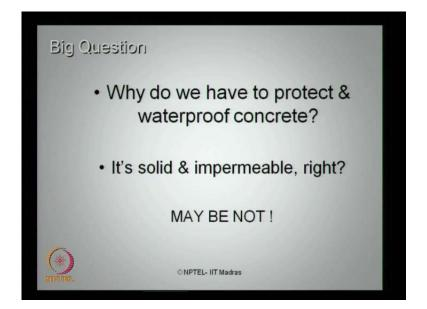
It is a big question that why do we have to protect and waterproof concrete? Because, it is solid and impermeable; if that is a case, if you understand it is impermeable and solid and integrable then there is no need to protect it, but it is not true; it may not be always true. Concrete is porous and permeable.
