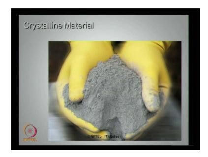
Now, the question comes, what do we understand by crystalline material? The photograph shows you here is a larger view of a crystalline material which is been held in the hands of an engineer. So, the larger view shows the further fineness of this material, which will be used as one of the ingredients to fill up the voids in concrete and making it impervious.
