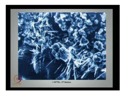
So, it is gets initiated which you see a photograph here. So, the crystalline formation have started happening in various locations. Ladies and gentlemen, remember, it is the permanent formulation which sticks on to the pores of the concrete structure.
