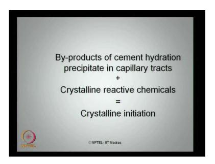
By-products of cement hydration precipitate in capillary tracts when added with the crystalline reactive chemicals results in what we see here as a crystalline initiation.
