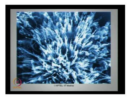
Now, you can see here the pores are completely fully occupied and permanently closed, because of the formation of this permanent crystalline structure which is actually a reaction happening with the chemical adhesive presents in the concrete with that of the crystalline material.
