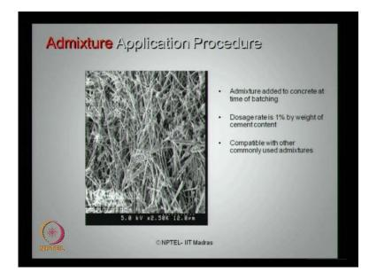
So the crystalline formation basically has admixture added to concrete at the time of batching itself. The dosage rate is about one percent by weight of cement content used in
