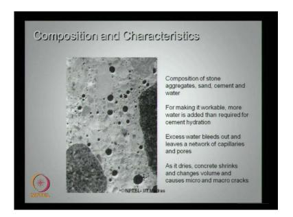
Let us quickly look at the composition and characteristics of concrete. We all understand we are civil and structural engineers, we know the importance and the method by which the concrete is manufactured or made for the construction sites. It is actually a composition of a stone aggregates, sand, cement and water. Now for making it workable, more water is added then required for cement hydration.
