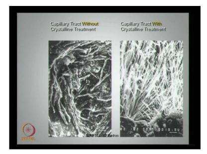
If you look at the photograph of capillary tract without crystalline treatment, and the capillary tract with crystalline treatment, you can see a phenomenal difference which has been shot in a close view of a scan electron micro scope. This shows me that the
