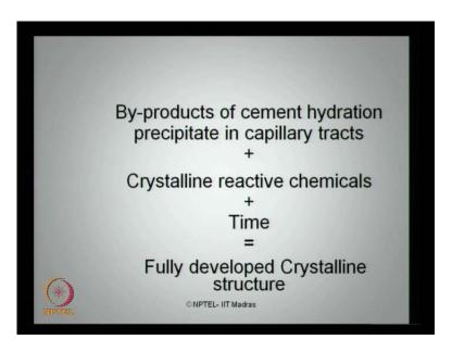
Further, the by-products of cement hydration precipitate in capillary tracts when added to the crystalline reactive chemicals will yield plus the time will yield a product which is seen now here, which is called fully developed crystalline structure.
