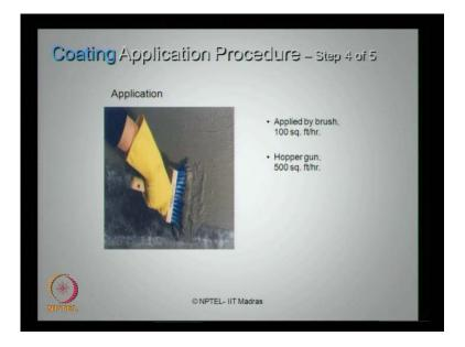
Once the mixture is prepared, and the surface is wetted and surface is prepared and ready for application then applied by a brush, the approximate coverage is hundred square feet an hour. You can also do an hopper gun application which will cover a larger area which is approximately out of 500 square feet an hour.
