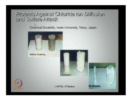
Now, the question comes, how does it protect against chloride ion diffusion and sulfate attack. The chemical durability is been tested in Iwate university, Tokyo, Japan. And look at this figures, where before soaking and after five weeks and after ten weeks what is been the state of presence of art of the cylindrical specimens which has tested in literature, to check for the chloride ion diffusion and sulfate attack on concrete.
