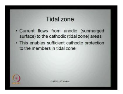
Current flows from anodic, which is submerged surface to the cathodic which is tidal zone in this areas in sea environment. This enables sufficient cathodic protection to the members in tidal zone automatically. This is caused, ladies and gentlemen, because the differential aeration present or because of formation of marine growth in the regions which are immersed below and not in the regions where as a tidal zone.
