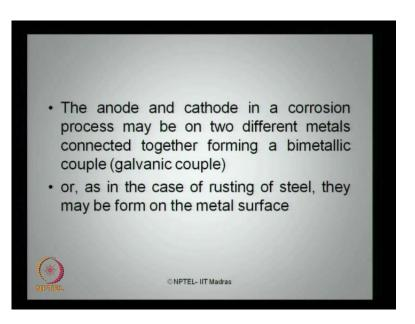
The anode and the cathode in a corrosion process may be on two different metals, which are connected together which can form what we understand as a bimetallic couple, which is otherwise referred as galvanic couple in the literature. Or on the other hand, in the case of rusting of steel, they may be forming on a metal surface itself.
