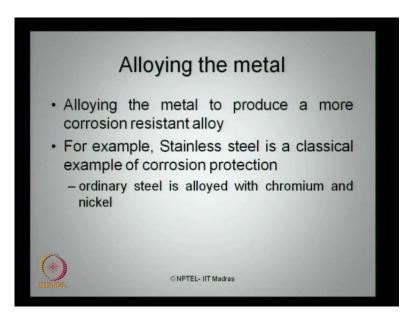
The second methodology by which we said is alloying the metal. So, you can alloy the metal to produce a more corrosion resistant alloy. There are significant examples available which we will be discussing now, for example, stainless steel is a very classical example of corrosion protection alloy which is an alloyed of ordinary steel with chromium and nickel. So, this alloy of chromium and nickel improves the conditioning of the original steel, and makes it corrosive resistant.
