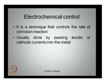
You can also control the electrochemical reaction happening which is also responsible equally for a corrosion process. Electrochemical reaction control is a technique, which control the rate of corrosion reaction. It is usually done by passing an anodic or cathodic current inside the metal.
