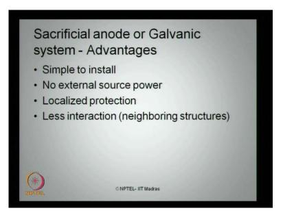
Whereas, as compared to the sacrificial anode or galvanic system, there are advantages, it is very simple to install, no external source power is required, localized protection is very highly effective and immediately available on float out, and less interaction with a neighboring structures.
