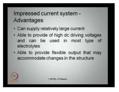
Alternatively, if we talk about impressed current system, it is having certain merits as listed below. Can supply relatively a larger current, therefore effective monitoring of control mechanism is highly feasible if you use impress current mechanism. It is able to provide high DC driving voltages and can be used in most type of electrolytes. It is able to provide flexible output; therefore it may accommodate respective changes in the structural members.
