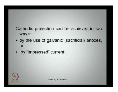
A Cathodic protection can be achieved in two methods. One - can use galvanic anodes, which we call as sacrificial anode technique. Or can use impressed current method, which we call as impressed current technique.
