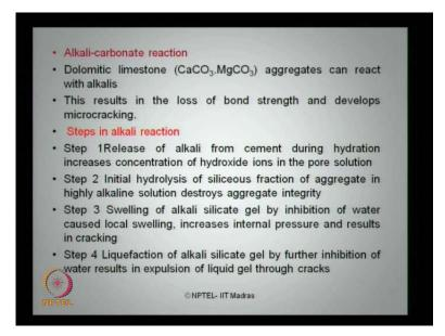
If you look at the alkali carbonate reaction present in concrete which is subjected to marine environment, the dolomitic lime stone aggregates can react with alkaline. This results in the loss of bond strength and develops what we call micro cracking in the concrete structure. The steps in alkali reaction can be seen as follows; as a first step release of alkali from cement during hydration increases concentration of hydroxide ions in the pore solution.
