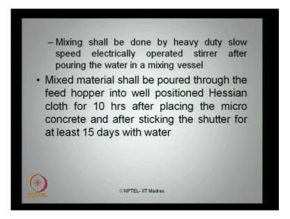
Mixing should be done by heavy duty, slow speed, electrically operated stirrer after pouring the water in the mixing vessel. Mixed material should be poured through feed hopper system into the well position hessian cloth for 10 hours after placing the micro concrete and after sticking the shutter for at least 15 days with water.
