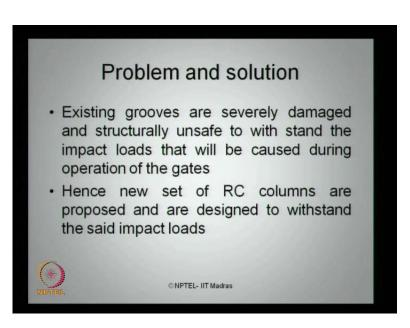
So, the problem what you just now saw is existing grooves are severely damaged and they seems to be structurally unsafe because they cannot withstand the impact loads, which are posed by the gate when the gate is being under operation. Hence, new set of reinforced concrete columns are propose in the design and the design to withstand the said impact loads caused by the gates.
