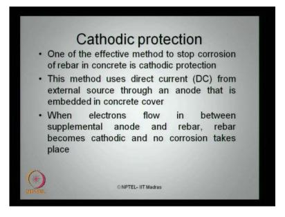
Cathodic protection forms a very major role in such kind of treatment, one of the effective methods to stop corrosion of reinforcement bar in concrete is cathodic protection. This method uses direct current from external source through anode that is embedded in concrete cover. When the electrons flow in between the supplemental anode and rebar, rebar becomes cathodic and therefore, it is protected because no corrosion takes place in the reinforcing bar.
