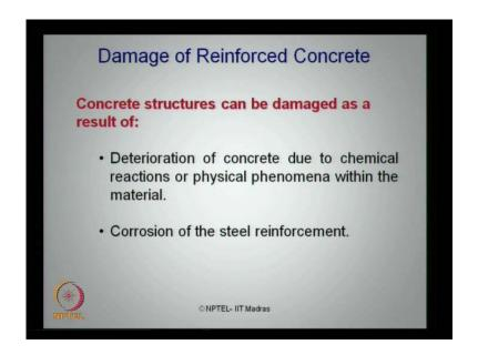
When you talk about damage of reinforced concrete ocean structural systems, there are very interesting points to be understood as far as concrete as a construction material is concerned. Concrete structures can be damaged as a result of either deterioration of concrete due to chemical reactions or physical phenomenon within the material. The second major issue is that the reinforcement, which is embedded in concrete, also receives a corrosive attack, because of the marine environment.
