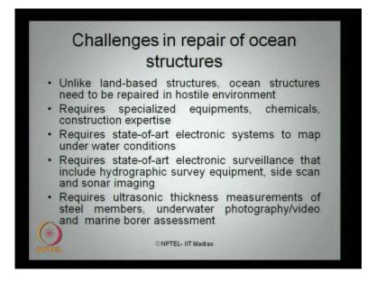
What are the challenges which are generally posted, while you attempt a repair on ocean structure? Unlike land based structures, ocean structures need to be repaired in coastal environment because these kinds of structures mostly have less or remote access to land. It also requires specialized equipments, chemicals and construction expertise to carry out repair with these kinds of structural systems.
