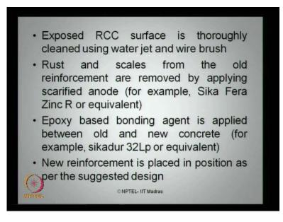
The exposed RCC surface is then thoroughly cleaned using water jet and the wire brush. Rust and scales from the old reinforcement are removed by applying scarified anode, which is for example, can be a Sika Fera Zinc R chemical compound or equivalent. Epoxy based bonding agent is then applied between the old and new concrete for example, Sikadur 32 Lp or equivalent can be used for such kind of applications. New reinforcement is now placed in position as per the suggested design.
