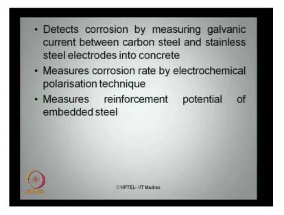
It detects corrosion by measuring the galvanic current between carbon steel and stainless steel electrodes with their embedded into concrete, it measures the corrosion rate by electro chemical polarization technique, it measures the reinforcement potential of the embedded steel.
