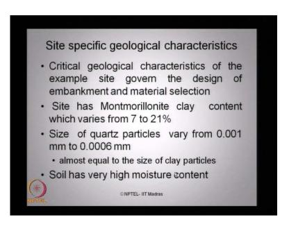
Now the question comes, what are those the sites specific geological characteristics, which generally govern these kind of design and construction methodology of embankments to prevent advancement of sea into offshore. The critical geological characteristics of the example site what we saw in the photograph govern the design of embankment as well as material selection for construction of embankments. The site has
