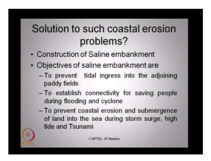
What are the solutions for such coastal erosion problems? The primary solution for coastal erosion problem can be construction of an embankment. Now we have a point here to say that one can also plan to construct what we called a saline embankment. Now
