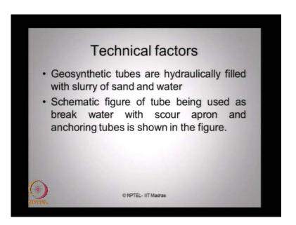
Now let us see those technical factors, which will govern or which will show advantages of using new materials like geotubes for coastal protection structures. Geo synthetic tubes are hydraulically filled with slurry of sand and water. The schematic figure of tube being used as breakwater with scour apron and anchoring tubes will be shown in to a following figure.
