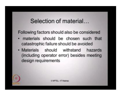
In addition, ladies and gentlemen, following factors should also be considered. Materials should be chosen such that the catastrophic failure should be avoided. Materials should withstand hazards including operation error besides meeting the design requirements.
