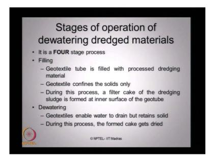
There are different stages of operation when you want to carry outing dewatering of dredge material. It is a four stage of process as now understand. The first stage is filling
