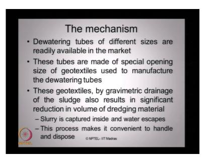
Let us quickly see how this mechanism works. The mechanism consists of placing dewatering tubes of different sizes, which are readily available in the market. These tubes actually are made of special opening size of geo textiles which are used to manufacture the dewatering tubes. These geotextiles, by gravimetric drainage of the sludge also results in significant reduction of volume of dredging material. However, you
