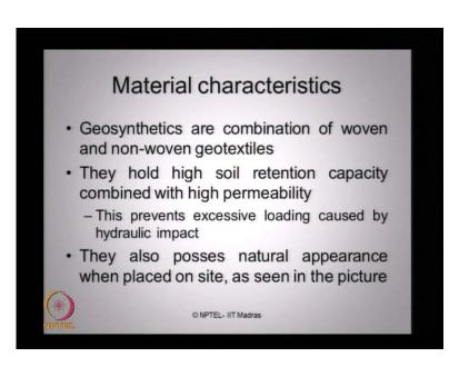
Let us quickly look at the different material characteristic, which has been used in modern construction practice for a coastal protection structure. Geo synthetics are combination of woven and nonwoven geo textiles. They actually hold a very high soil retention capacity combined with very high level of permeability. This prevents excessive loading caused by hydraulic impact on such structure. They also possess natural appearance when placed on site as you seen in the photograph.
