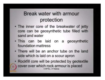
Let us look at the breakwaters with armour protection which is being recently attempted with geo synthetic tubes. The inner core of the breakwater of jetty can be geo synthetic tube, which is filled with sand and water. This can be laid on a geo synthetic foundation mattress, they drain away they eroded water. There will be an anchor tube on the land side which is laid on a scour apron. The rock fill core will be protected by the geotextile cover over which the rock armour is placed.
