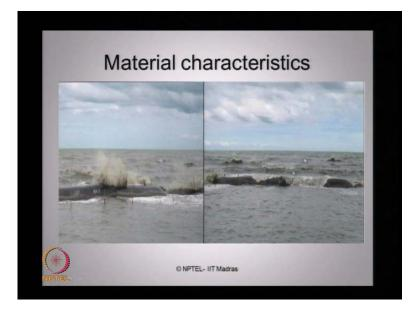
Now I got geo synthetic tubes, which has been placed on a site and they actually merged with elevation sea surface what you see in the gray color. So they get amalgamated in nature, so that you may not use in notice then the artificial layer which has been provide as the protection layer for the coastal site as they get merged with the sea states.
