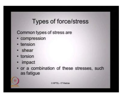
There are different types of forces and stresses that act on material, when they are housed in construction for offshore structure. Common types of stress which are see in material are the following - compression stresses, tensile stresses, shear, torsion, impact or a combination of these stresses such as fatigue.
