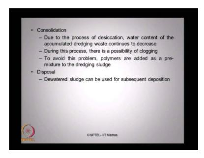
In third stage, we have a consolidation process where due to the process of desiccation, water content of the accumulated dredging continues to decrease from the geotube. During this process, there is a possibility of clogging. To avoid this problem, there are certain polymers are added as a pre-mixture to the dredging sludge, before the sludge is filled in geo synthetic tubes. Then the fourth stage is disposal of this dewatered sludge, which can be used for subsequent deposition.
