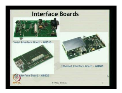
Let us talk about the detail of interface boards, which are used for this kind of sensor networking. It has serial interface board MIB 510 or you can also use USB interface board which is MIB 520 which can be connected to the USB card. It also has Ethernet interface board which can be connected data acquisition directly to the intranet facilities.
