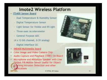
If you look at Imote 2 wireless platform, the photograph of Imote 2 looks as we show below. It contains an ITS-400 sensor board, which has got dual temperature and
