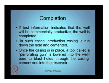
If the test information indicated that the well is commercially productive, then the well should be complete. So, what you understand by completion, then in such cases production casing is run down the hole and then cemented. Once the casing is in place, a tool called a perforating gun is lowered into the well bore to blast to blast holes through the casing cement and into the reservoir.
