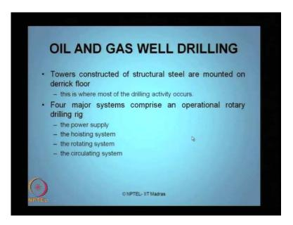
Towers constructed of structural steel are mounted on derrick floor. This is where most of the drilling activity occurs. Four major systems comprise an operational rotary drilling rig. Let see what they are. The power supply system, the hoisting systems, the rotating systems, and the circulating systems are four vital compliment of what we called as rotary drilling.
