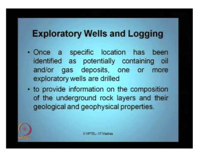
Once a specific location has been identified as potential space, which contain oil and gas deposits then one or more number of exploratory drills are drilled. To provide information on the composition of the underground rock layers and their geological and geophysical properties, surveys are carried out.
