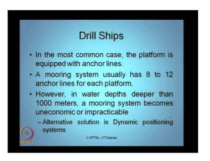
In most common case, the platform is generally equipped with anchor lines. A mooring system are generally order has above 8 to 12 anchor lines for each platform. However, in water depths deeper than 1000 meters, a mooring system becomes uneconomical or impracticable. Now one may wonder what you do, if you want go for drilling beyond 1000 meters, obliviously alternating solutions is dynamic positioning systems.
