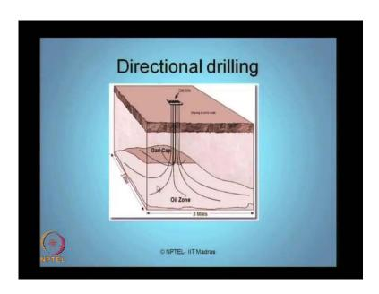
What you understand by directional drilling? Ladies and gentlemen, as you see here in this figure, if you want to do a drilling actually from the moon pool of a ship. I said the moon pool should located exactly above the drilling hole, I prefer to drilling vertically down, but sometimes we have to also extent the drilling not exactly vertical but also have possible lateral direction to touch as far as possible the boundary of the hydrocarbon traps.
