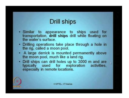
Drill ships have similar to the appearance to ships except that drill ship drill while floating on sea surface. During operation, the drilling takes place through a hole that we call as moon pool. The large derrick is mounted permanently above the moon pool, which is similar to that of land rig. Drill ships can drill holes up to 3000 meter deep, and are typically used for exploration drilling. Remember the drill ships are never equipped or never adapted for production drilling.
