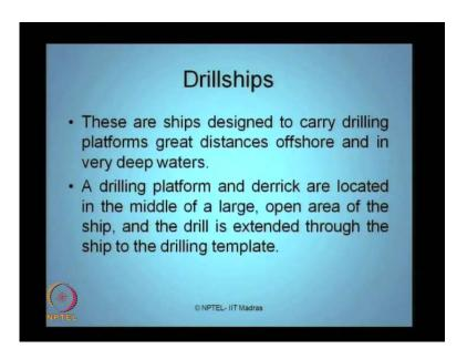
Drills ships are designed to carry drilling operations are greater distance offshore and in very deep waters. A drilling platform and derrick will be located in the middle of a large, open area of the ship, the remaining recollect terminology which is middle, large, open area in the ship which a called as a moon pool. Moon pool is nothing but is hole extended through the hull through which the drilling rises will be placed through the hull to the drilling template.
