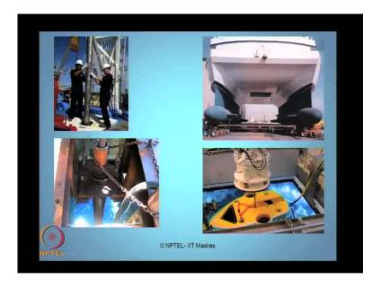
These are some of photographs which show you the details of moon pool. You can see here moon pool is nothing but hole, which is driven the top of the hull which passes through and through. You can see here the hole through and through, you can see the waterbed here, and you can see the sea surface here. This is the very specific drilling mechanisms or the drilling rises are connected in pieces has the drilling progress deeper and deeper.
