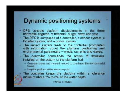
What are dynamic positioning systems? DPS is basically is a control which activate the control systems of the platform which control essentially a displacements in three
