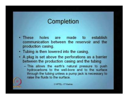
These holes are made to establish communication between the reservoir and the production casing. Tubing is then lowered into the casing. A plug is set above the
