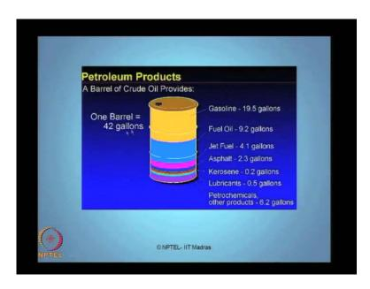
Let as look into some basic concept of oil drilling. Start form a petroleum product, petroleum product comes actually a barrel of crude oil, which is composition of 19.5 gallons of gasoline, 9.2 gallons of fuel oil, 4.1 gallons of jet fuel, above 2.3 gallons of an asphalt, above 0.2 gallons of kerosene, and above 0.5 gallons of lubricants and above 6.2 gallons of other products. So it comes in a barrel which is approximately base 42 gallons.
