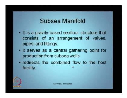
Let us talk about another important component of the subsea system, which is subsea manifold. What is the subsea manifold? It is actually a gravity based seafloor structure.
