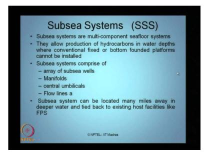
Subsea systems briefly are called as SSS. Subsea systems actually on multi-component sea floor systems; the moment is a multi-component one would like to know the different components that are present in a sea floor system. Essentially let us look at the function
