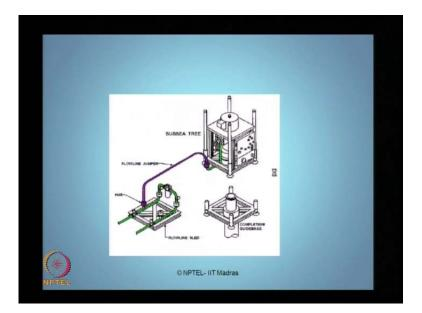
The other figure shows how the subsea tree is connected to the hub using what we called a flow line jumper.
