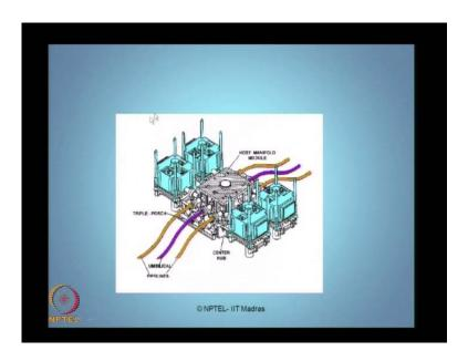
We can see a typical figure of a template which contains umbilicals. Umbilicals of given different color; this can be either different conduits, can be even pipes, can also have what we called pipelines which are given in different color. We have center hub, which connects the host manifold module to that other different facility.
