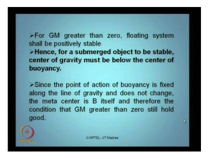
For G M greater than zero, the floating system shall be positively stable. Hence, it is very simple to summarize for a submerged object to be remain stable the center of gravity must lie below the center of buoyancy. Since, the point of action of buoyancy is fixed along the line of gravity and does not change the meta center is B itself and therefore, the condition that G M greater than zero still holds good in our argument.
