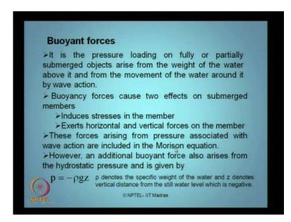
Let us look into the other type of force what we call buoyant forces. It is the pressure loading on fully or partially submerged objects arise from the weight of water above it and from them moment of water around it around it by wave action. Buoyancy forces cause two effects on submerged members. One, it induces stressin the member, two it exerts horizontal and vertical forces on the member.
