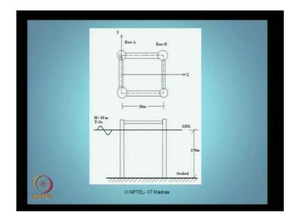
So, you got 4 members, cylindrical members and 4 quantum members, which are spaced 10 meter interval both along X and along Y. So, the depth is 150 meter water depth. So, I want you to compute the forces on all the members using Airys linear wave theory.
