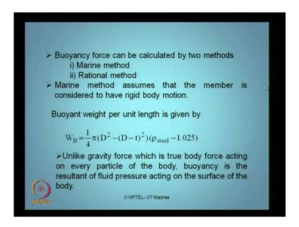
The buoyancy force can be computed by two methods. One is what we call as a marine method; other is what we call as a rational method. The marine method assumes that the member is considered to have rigid body motion. In that case the buoyant weight per unit length of the member is given by this equation. Unlike the gravity force which is truly a body force acting on every particle of the body, buoyancy is resultant of fluid pressure acting on the surface of the body.
