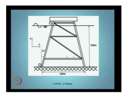
This is the problem where awarded, inclined member, the member is inclined 30 degree to the vertical, this is 100 meters. So, I want you so find out the forces of the member 1 2 as shown in the figure here.
