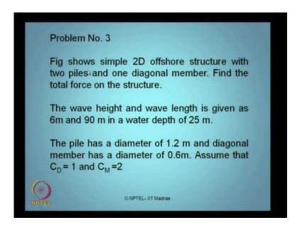
Let us see problem number 3. Again, there is a figure shown of a two dimensional offshore structure with 2 piles and 1 diagonal member, find the total force on the structure, the wave height and wave length are given as below, the pilled diameter has a member of about 1.2 and the diagonal member has a diameter of 0.6 meter.
