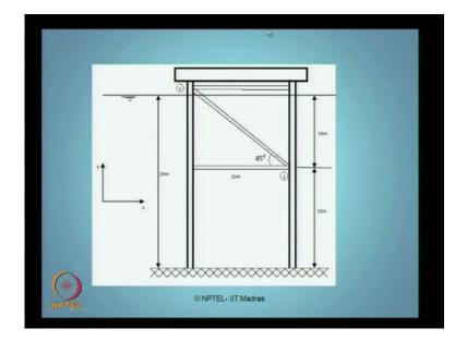
This is the figure, this the member 1 and member 2. I want you to determine the force on the diagonal member 1 2. So, I given all the dimensions of the member, the water depth, the water (( )), estimate the forces. I think you will be able to solve this problem with the help of equations given to you. We can use any appropriated wave theory, there is no problem.
