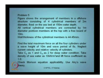
Problem number 5 shows the arrangement of the members in an offshore structure consisting of 4 cylindrical members of 2 meter diameter fixed on the sea bed at 150 meter water depth. All the vertical cylindrical members are connected by 1 meter diameter pontoon members with a free board of 10 meters, wall thickness is given as 44.5 millimeter, find the total maximum force on all
