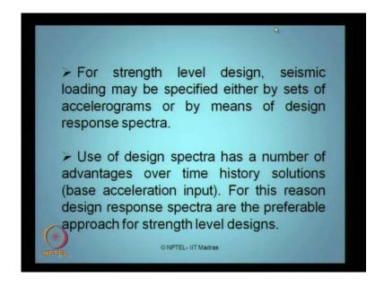
For the strength level design, seismic loading may be specified either by sets of accelerograms or by means of design response spectra. The use of design response spectra has a number of advantages over the time history solutions which is based on the base acceleration input. For this reason the design spectra are generally preferred for strength level designs in offshore structural designs.
