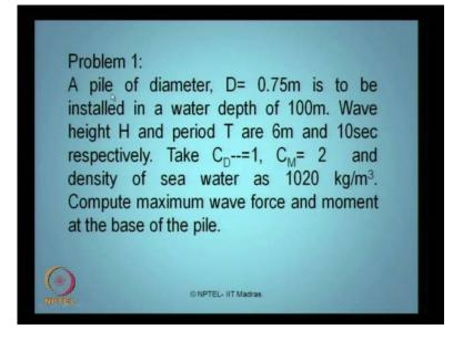
Let say problem number 1 I have a pile of diameter 0.75 meter which is to be installed at a water depth of 100 meters, the wave height and the wave period are taken as 6 meter and 10 second respectively. Take C D and C M as 1 and 2 respectively and take the density of sea water as 1020 kg per cubic meter. What I want you is very simple, compute the maximum wave force and the moment at the base of this pile?
