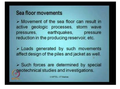
The other kind of force which acts on members of offshore is sea floor movement. The movement of the sea floor can result in active geologic processes, can activate storm wave pressures, it can cause what we call earthquakes, it cause pressure reduction in producing reservoir etcetera. Then the loads generated by such moments after the design of the piles and jackets of offshore structures. Such forces are determined by special geotechnical studies and investigations.
