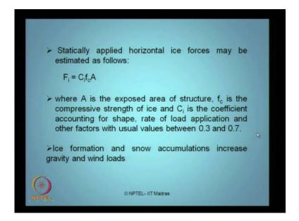
Statically applied horizontal ice force may be estimated from the given equation given here, where in this equation A is exposed area of structure, Fc is the compressive strength of ice and Ci is the coefficient accounting for shape, rate of loading application and other factors with usual values between 0.3 to 0.7 as seen in the literature. The ice formation and snow accumulations increase gravity as well as wind loads coming on the offshore platform.
