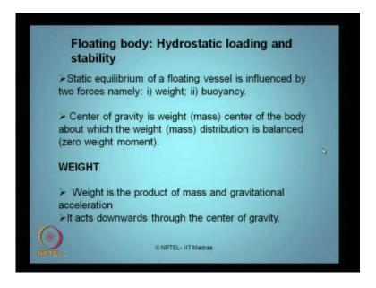
After understanding how to compute the wind forces and wave forces, now let us see how to understand what is the significant of hydrostatic loading and stability of a floating body. The static equilibrium of a floating vessel is influenced by two forces namely weight and buoyancy. The center of gravity is weight or mass center of a body about which the weight distribution or the mass distribution is balanced. We call this as zero weight moment.
