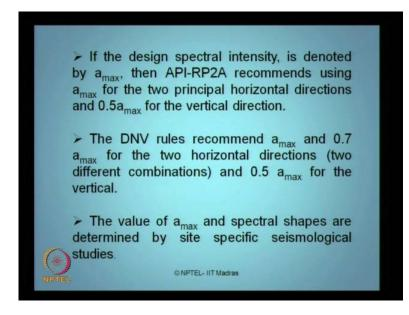
In the design spectral intensity is denoted by a max then international codes like APRP2A recommends using a max for two principal horizontal directions and 0.5 of a max for the vertical
