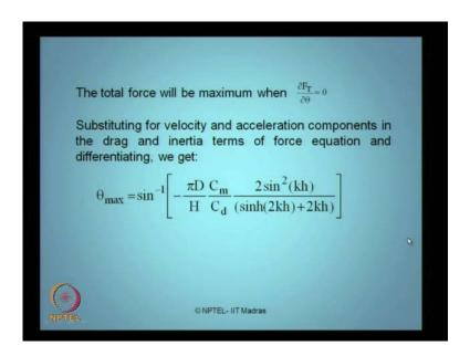
The total force will be given when this equation is satisfied so by substituting the velocity and acceleration components in the drag and inertia terms of the force and differentiating it I can find the maximum angle at which the force can remain at maximum. So, I will compute the maximum angle, substitute this back in the force equation and try to find the maximum force in the given member.
