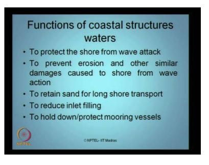
Let us ask a fundamental question, what are all various functions of coastal structures constructed in waters? To protect the shore from wave attack, to prevent erosion and other similar damages caused to the shore from the wave action, to retain sand for long shore transport, to reduce inlet filling, to hold down protect mooring vessels in position.
