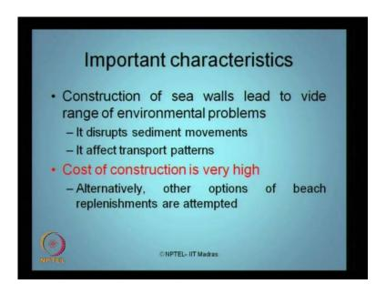
There are important characteristics of a sea wall, which we require to understand. The construction of sea walls leads to wide variety of environmental problems. For example, it disrupts the sediment movements, it affect the transport patterns of the sediment. The cost of construction of sea walls is very high, so it is consider as one of the negative or
