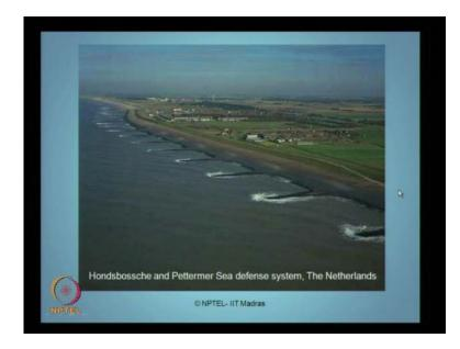
This photograph shows the Hondsbossche and Pettermer sea defence system constructed at Netherlands; you can see here a very long coast line has been protected by construction of sea dikes.
