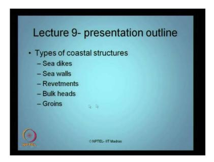
We will talk about different types of coastal structures, which are constructed for various purposes. For example, in this lecture we will discuss about, sea dikes, sea walls, revetments, bulk heads and groins.
