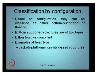
So, we will move forward. Llet us talk about classification by configuration. The functional aspect is different. I want to now classify the platforms based on the geometric configuration. They can be either classified as bottom-supported or floating. Bottom supported means the platform can rest on sea floor.
