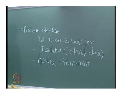
So, foremost condition for an offshore structure is? For any offshore structural systems, the foremost requirement which is dangerous is, it has no access to land which is openly available. So, they are isolated; what we call them as standalone systems. They are subjected to hostile environment. In case of any correction, any repair or any emergency, you want to attend but they are not readily accessible. So, this limits the number of installations to be very less.
