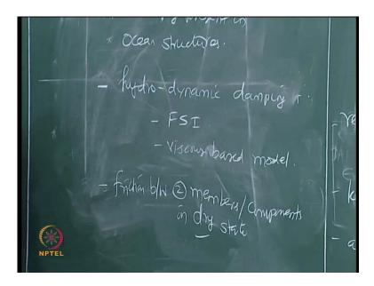
The inherent damping present in ocean structures is the following. One is, because of wave structure or fluid structure interaction, there is a component of hydrodynamic damping. This mainly arises from fluid structure interaction. I am just saying FSI and we already know, this is viscous, viscous based model because it depends on the velocity. The second kind of damping is also present in the system because of friction between two members' components in dry state.
