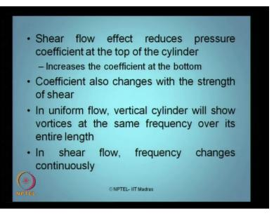
So, in the cylinder itself at the top the pressure coefficient decreases whereas the bottom it is increasing. So, there is a differential pressure set to the cylinder link itself the coefficient of course, changes with the strength of shear present in the fluid flow when the uniform flow cylinder will show vortices of the same frequency over the entire length of the cylinder keep the flow is very uniform of course, if the shear flow the frequency changes continuously.
