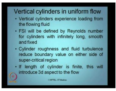
We look at the Vertical cylinders at uniform flow the Vertical cylinders experience loading from the flowing fluid again the fluid structure will again define Reynolds number for the cylinders provided the cylinders are consider to be infinitely long smooth and fixed. So, if you have got infinitely long smooth and fixed cylinders then you can always estimate the response of these members in a FSI region purely based on Reynolds number only the cylinder roughness and fluid turbulence.
