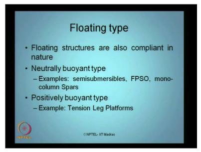
When we talk about the next type of configuration which is the floating type we already said floating type are also compliant in nature then in this case we can neutrally buoyant type structures like semisubmersibles, FPSO, and mono column Spars where as in also have Positively buoyant type where TLP understand the form is very interesting because the buoyant enormously exceeds the weight of the platform.
