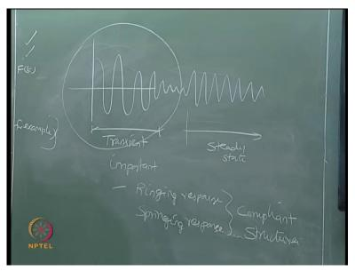
It can be a Transient response and then of course, it can be a Steady state response we already seen the categorically difference between the Transient response and Steady state response single degree freedom analysis in the last module. So, sometimes interestingly even the Transient response sector can also become important this can cost what we call Ringing response and Springing response essentially on complain structures.
