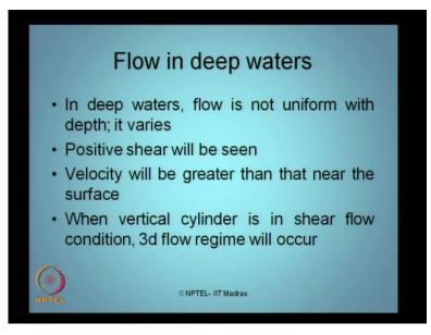
So, look at flow in deep waters the flow is not uniform with the depth it varies Positive shear will be mostly seen Velocity will be greater than that near the surface as you go deeper and deeper where vertical cylinders in shear flow condition then generate what we called 3d regime in the flow field.
