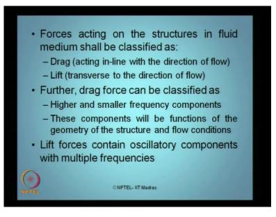
So, the Forces acting in the structure in the fluid medium can be further classified interestingly into two parts one is what we called as the Drag force which acting in line with the direction of flow the other is what we called a Lift force which transverse to the direction of flow (Refer Time: 31:26) variation of two parts we all know this.
