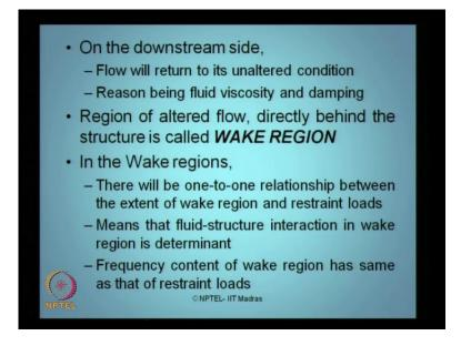
Frequency components I will talk about the fluid structure interaction when the wave train is skipping a member on the downstream side on the downstream side Flow will return to its unaltered condition after it interacts with the member after the flow pass the member.
