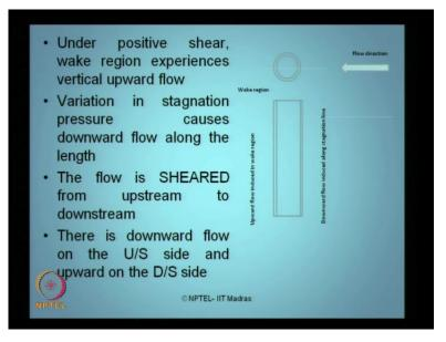
So, if you look at the wake region interestingly this may cylindrical member this may flow direction which is may flow direction if this may flow direction on the upstream side the flow is downward where as in the downstream side the flow is upward. So, the presence of member alters the flow field in the wake region like this I say just now said the again the member is what we call as a wake region. So, on the upstream side the flow is downward where as in the downstream side the flow is upward.
